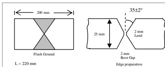
**Figure 1: Details of the Weld Configuration**
