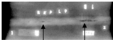
**Fig 2 – Lack of Penetration**
