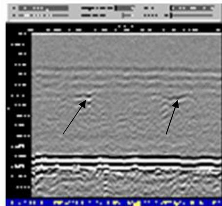
**Fig. 5 - UT Pulse echo (top) and TOFD image of Lack of Penetration (bottom)**
