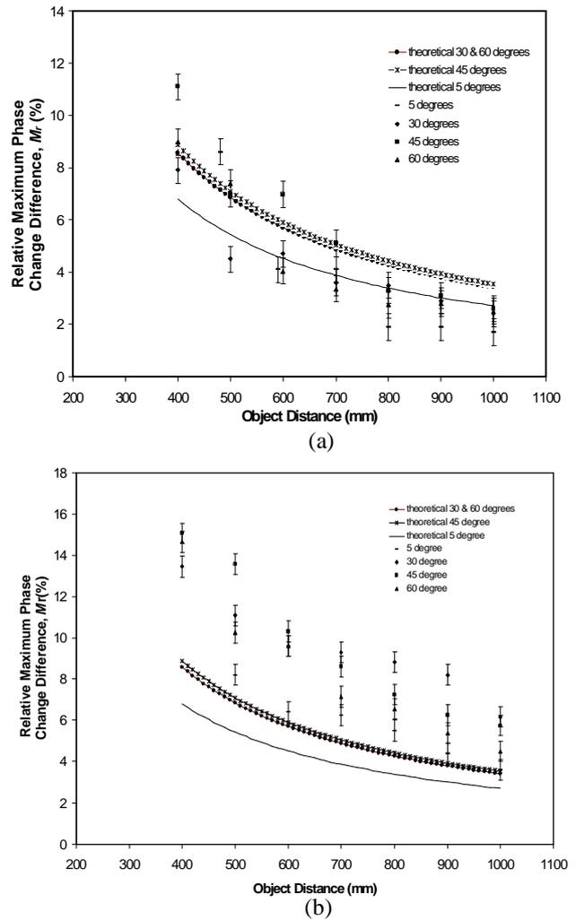
Figure 2: *Relative maximum phase change difference versus object distance for a different illumination angles, with a horizontal shears of (a) 5mm and (b) 15mm and illuminated area of 100mm x 30mm.*
