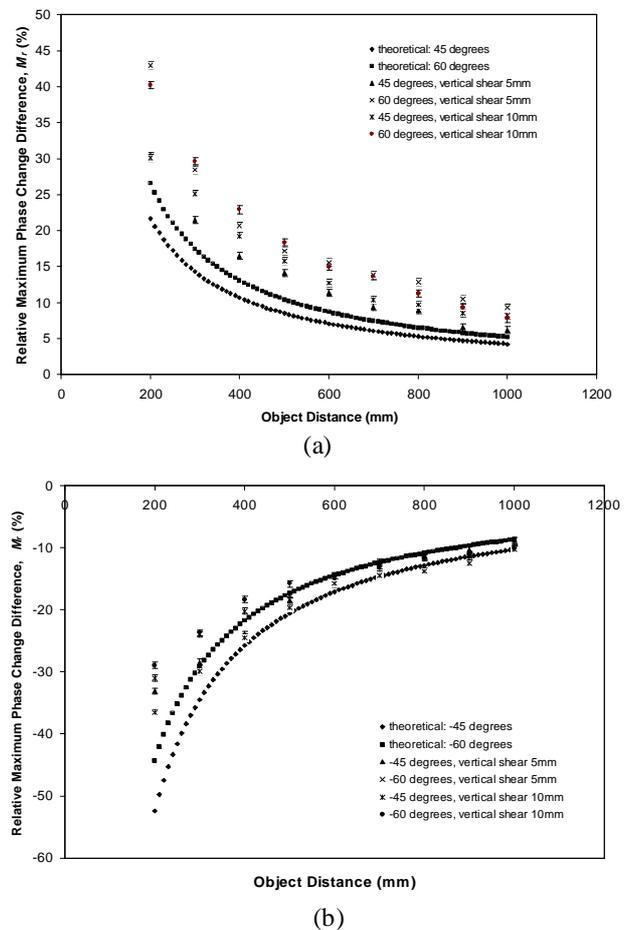
Figure 3: The relation of relative maximum phase change difference with the change of object distance (illumination curvature) for different shearing amount, the free end of the beam at right side relative to the camera axis, (a) positive illumination angles at  $45^\circ$  and  $60^\circ$ , (b) negative illumination angles at  $-45^\circ$  and  $-60^\circ$ .
