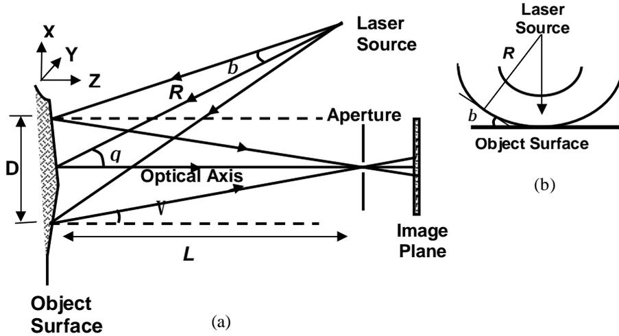
Figure 1: (a) Schematic representative of the optical path length on the inspected object surface, (b) Inclination of the curvature illumination wavefront on the object surface.
