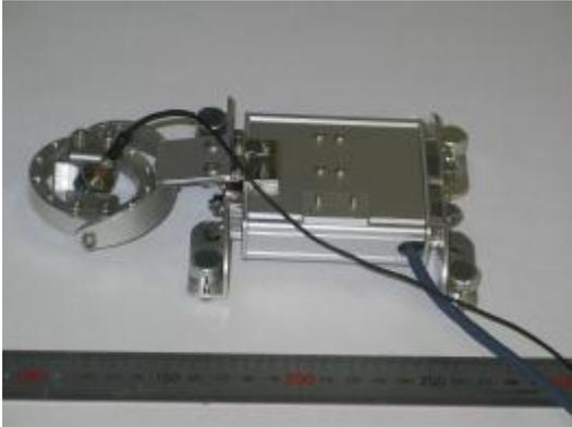
Figure 9: Portable X-Y scanner
