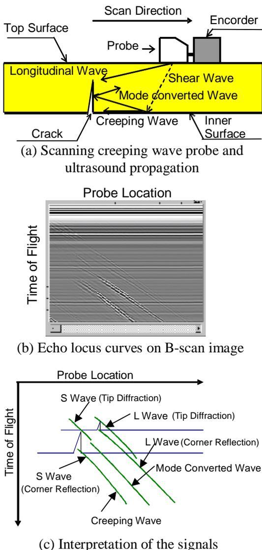
Figure 1: Relations between amplitude, time of flight and probe position
