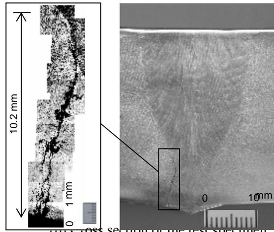
(b) Cross section of the test specimen with SCC
