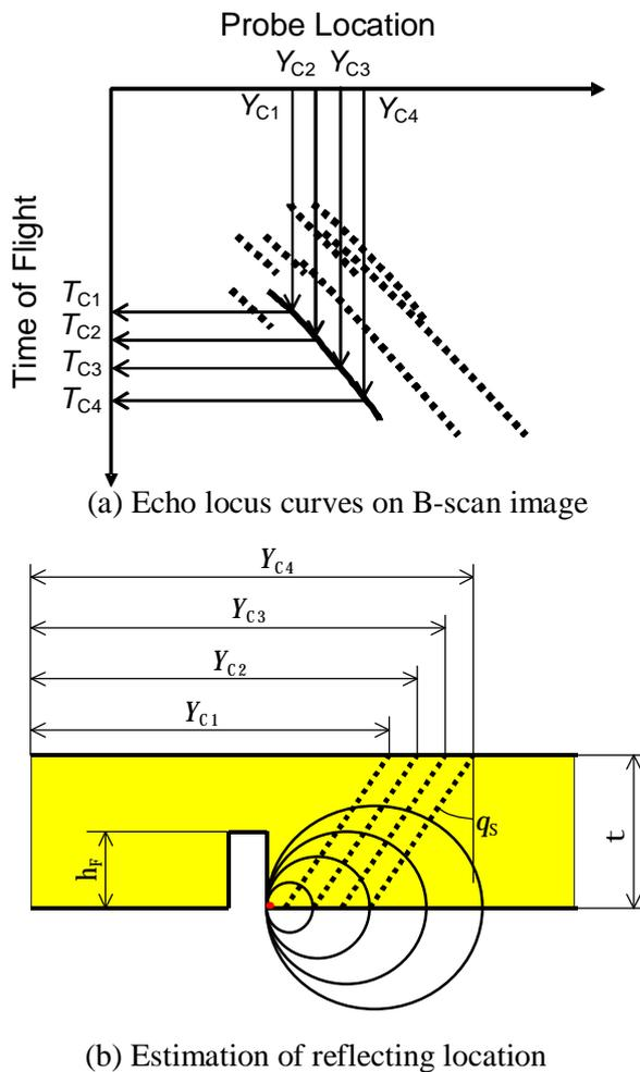
Figure 3: An example result of creeping wave technique
