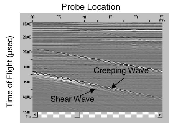
Figure 4: Separation of creeping wave signal and shear wave signal on locus curves
