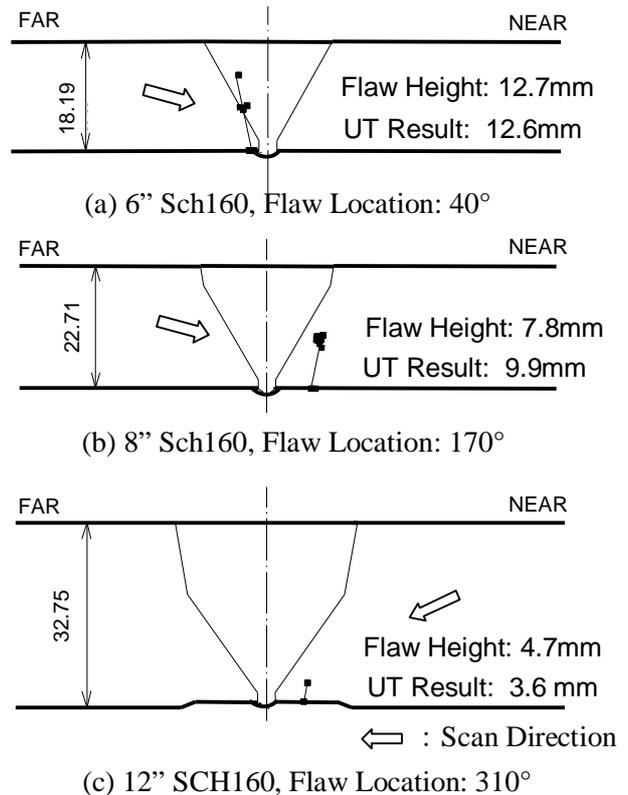
Figure 7: Results of flaw reconstruction on cross sectional view
