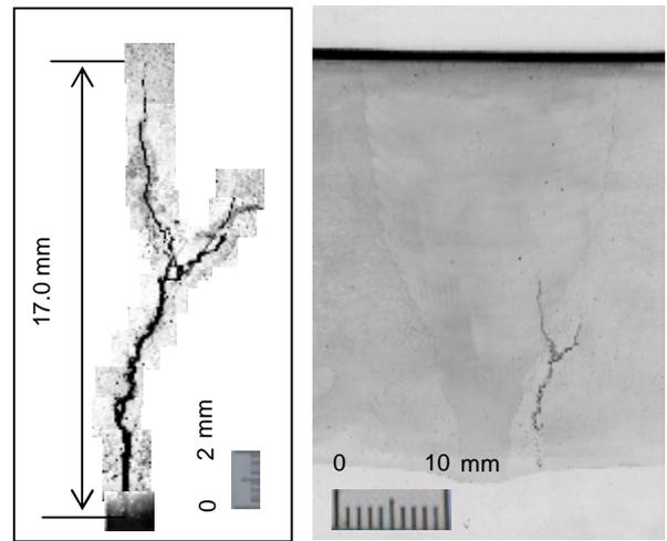
(b) Cross section of the test specimen with SCC
