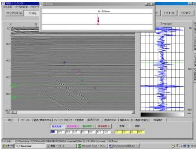
(a) Sizing result using creeping wave probe (SUS316, 600A)
