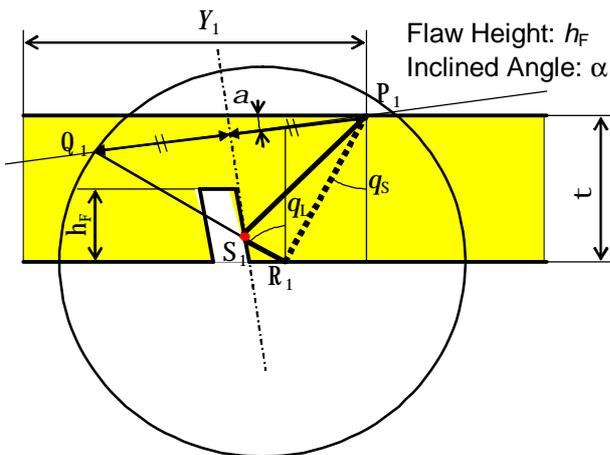
Figure 6: Mode conversion technique for the inclined flaw
