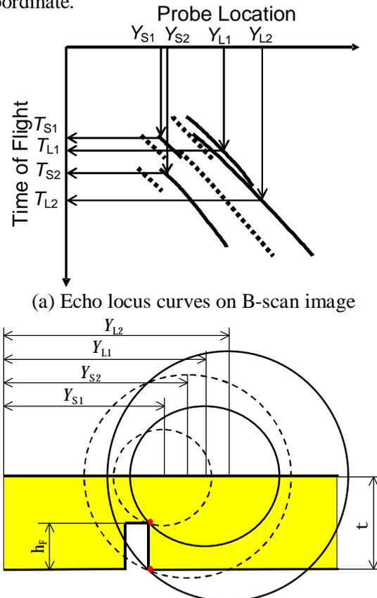
Figure 2: An example result of sizing technique using both longitudinal wave and shear wave
