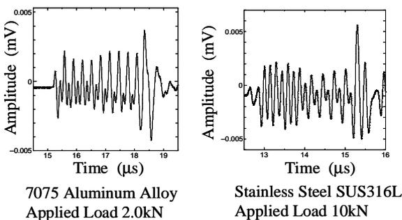
Fig.6 Typical waveform of each material
