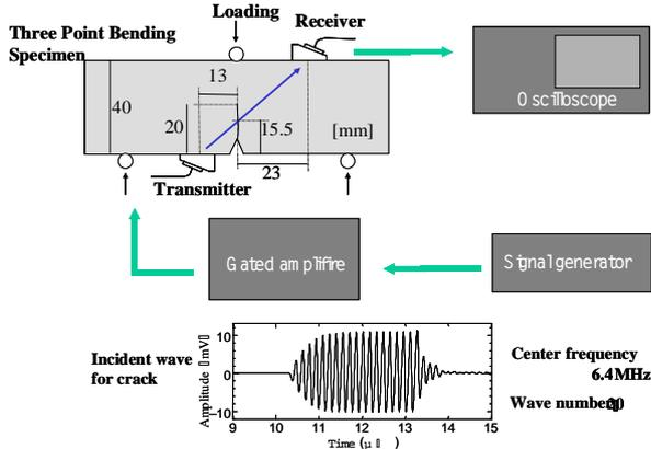
Fig.1 Nonlinear ultrasound measurement setup
