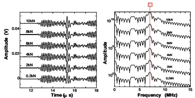
Fig.4 Waveforms due to applied load (Stainless steel SUS316L)
