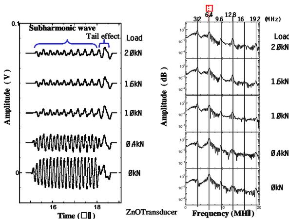
Fig.2 Waveforms due to applied load (Aluminum alloy A7075)
