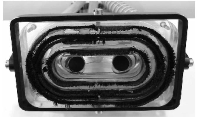
Figure 2 ACES™ dripless recirculating immersion scanning head<sup>1</sup>.
