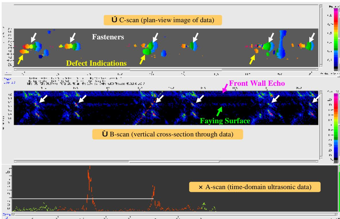
Figure 3. Data presentation for automated ultrasonic system.
