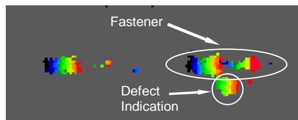
Figure 7 Typical mid-bore defect indication in depth mode C-scan.
