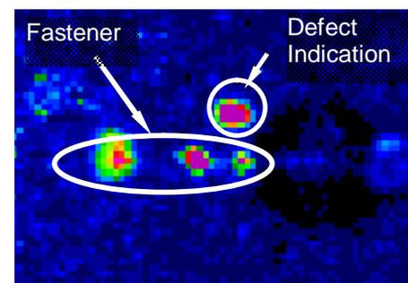
Figure 6 Typical corner defect indication in peak mode c-scan
