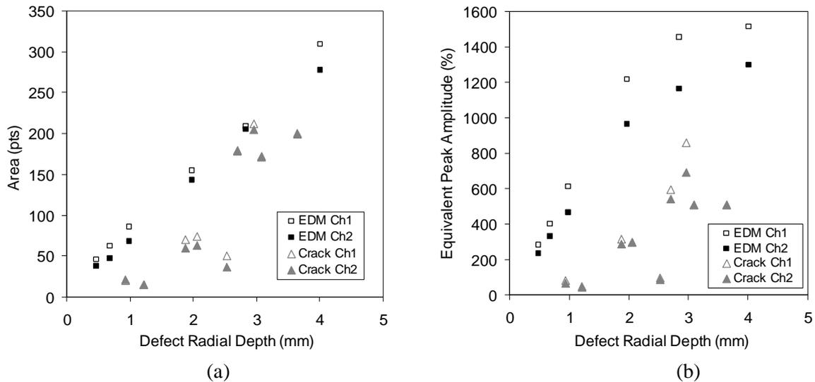
Figure 11. Ultrasonic response from corner fatigue cracks in specimens compared to corner EDM notch defects. (a) Area of indication above threshold, (b) Equivalent peak amplitude. [5]
