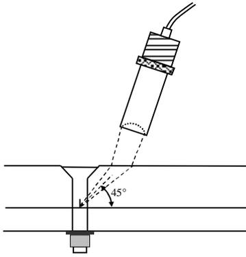
Figure 1 Schematic of 45° angle-beam shear-wave inspection using focussed immersion transducers
