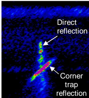
Figure 9 B-scan showing a typical large corner crack exhibiting both a corner trap reflection and a direct reflection. (Small corner cracks exhibit the corner trap reflection only.)
