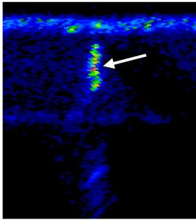
Figure 8 Direct reflection (arrowed) from a mid-bore crack in the B-scan
