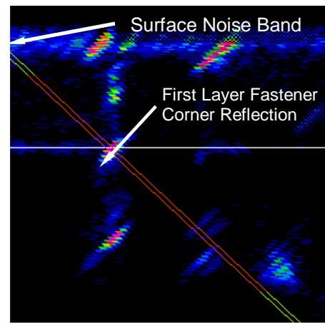
Figure 5 Fastener hole reflections in the B-scan
