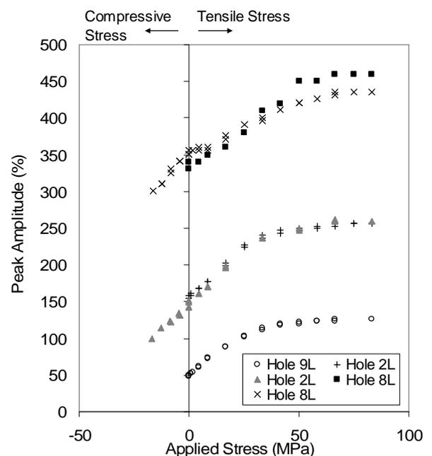
Figure 12 Ultrasonic response from fatigue cracks in specimens under an applied compressive and tensile stress.
