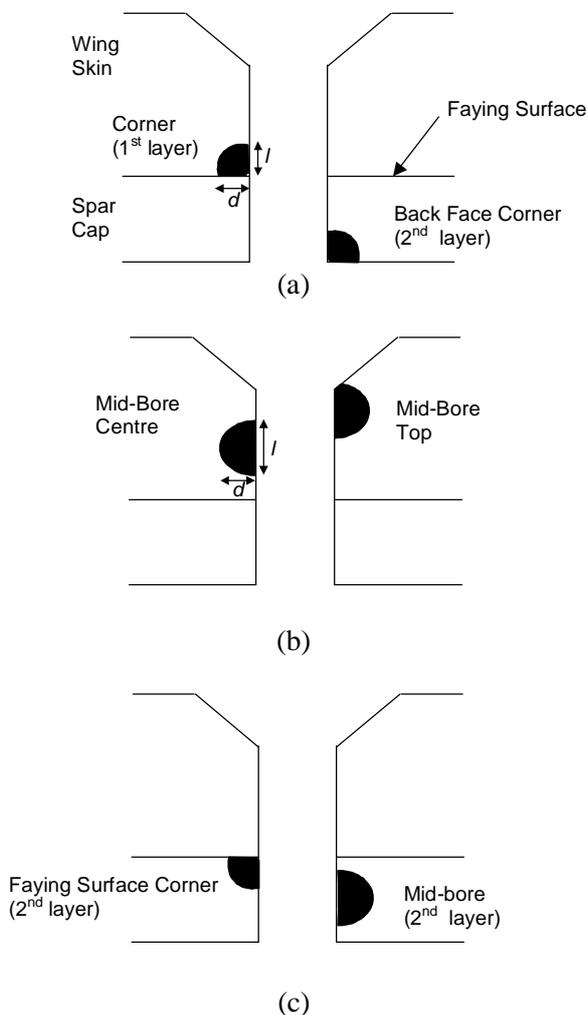
Figure 4 Schematics showing cross-section of fastener holes and the geometry of EDM notches inserted in test wing: (a) corner and back-face corner. (b) mid-bore centre and mid-bore top. These are distinguished according to their location at either the centre of the hole bore (centre) or immediately under the countersink (top). (c) faying surface corner and second-layer mid-bore. All EDM notch defects were nominally half- or quarter-penny in shape.
