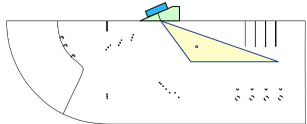
Fig. 4 Position A, Angle scanning on a 2 mm SDH
