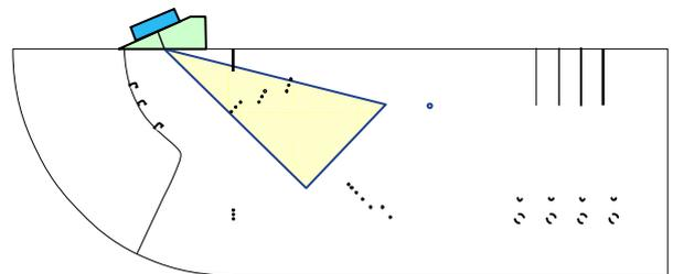
Fig. 5 Position B, Angle scanning on groups of square notches
