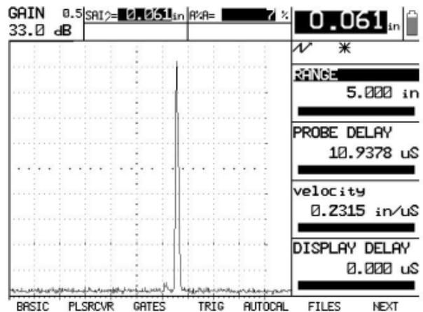
Fig. 14 Position C with conventional UT
