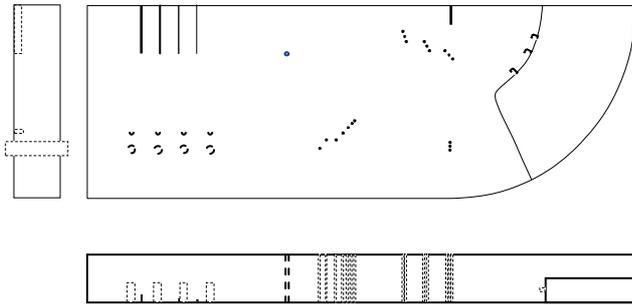
Fig. 2 Aluminum test block with groups of artificial flaws
