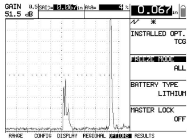
Fig. 18 Position E with conventional UT
