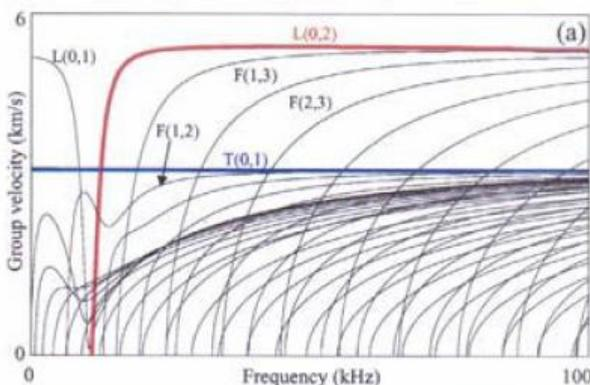
Figure 6: dispersion curves for 6 inch, schedule 40 steel pipe
