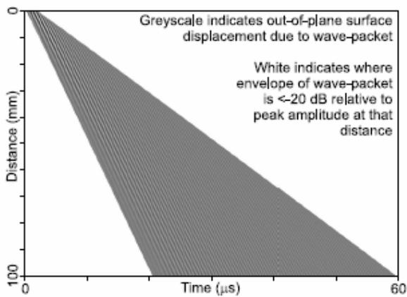
Figure 3: numerical simulation of the space-time map illustrating the dispersive propagation of the S0 mode in a 1-mm thick aluminum plate when the input signal is a 5-cycle hamming windowed toneburst with a centre frequency of 2Mhz
