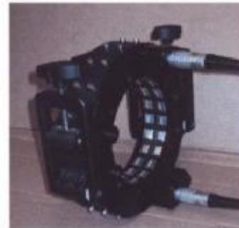
Figure 3: Transducer array for 8 inch pipe
