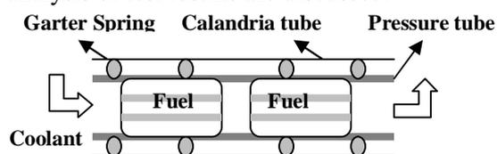
Figure 1: Simplified sketch of coolant channel
