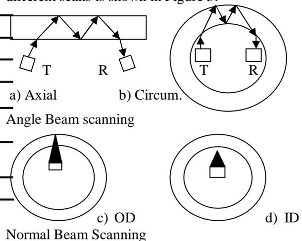
Figure 3: Angle & Normal Beam scans
