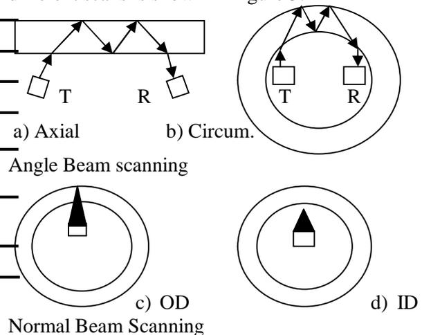
Figure 3: Angle & Normal Beam scans
