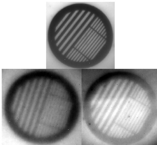
Figure 1: *Optical image (top), x-ray image using an Agfa MD-30 imaging plate (bottom left) and an x-ray image using one of our plates*
