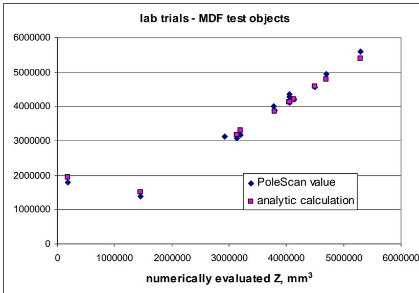
*Figure 6: comparison of section moduli. The objects range in diameter from 340 to 380 mm, both solid and with holes of 200 to 300 mm diameter. The squares are calculated from the formulae for circles, and the diamonds are from PortaScan analysis. The horizontal values are from numerical calculations.*
