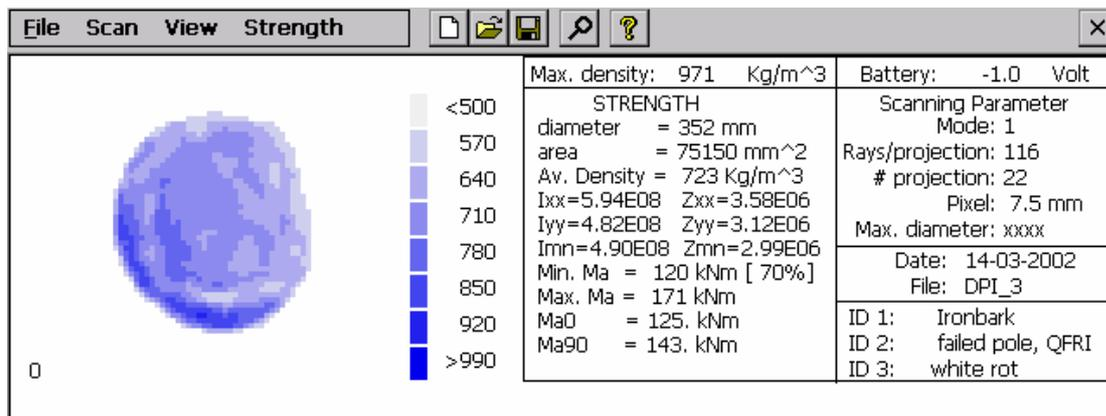
Figure 2: PortaCAT example of pole cross section evaluation
