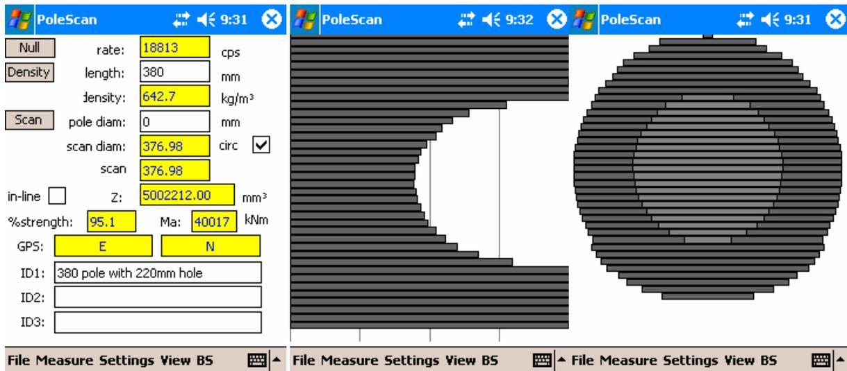
**Figure 5: PortaScan PDA screens: parameters (l.), average chord density (m.), reconstructed image showing centralised missing pixels (r)**
