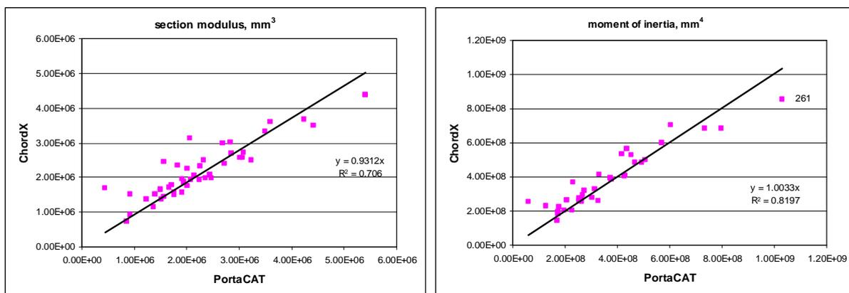
*Figure 7: comparison of moments of inertia and section moduli of real poles using PortaCAT data measured during EANSW 1998 trials reprocessed according to the PortaScan principle.*
