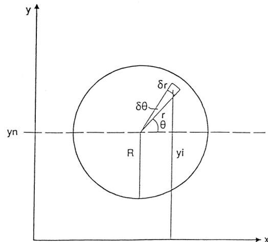
**Figure 1: section modulus calculation about neutral axis  $y_n$**
