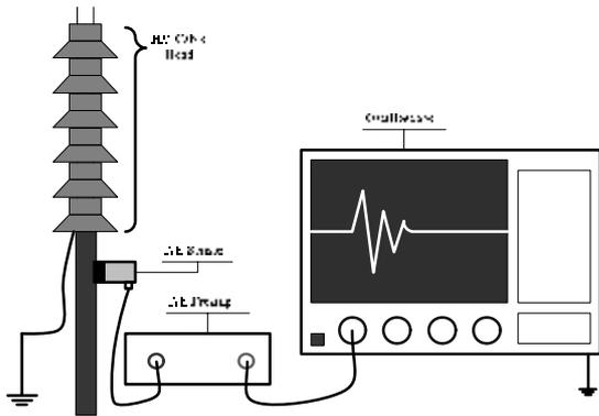
Figure 2 : *The acoustic emission measurement system.*
