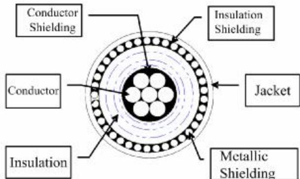
Figure 3 : *The base cross-sectional structure of power cable.*
