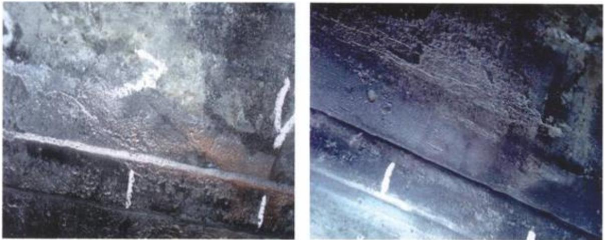
Figure 5. *Stress-corrosion with depth up to 5 mm located along longitudinal weld*
