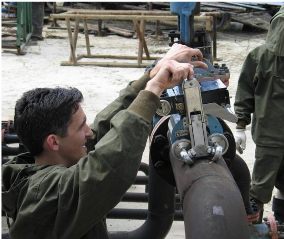
Figure 11. Scanner “SKM-T1”, inspection of pipe with diameter 168mm
