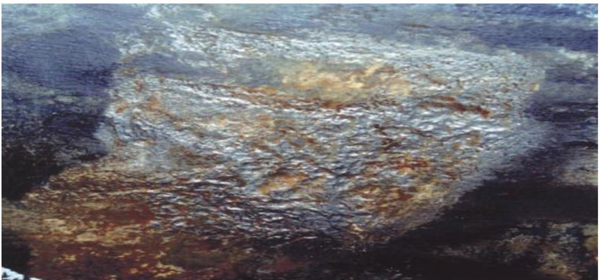
Figure 6. *General corrosion on the chemical stress concentrator (corrosion), depth 6 mm.*
