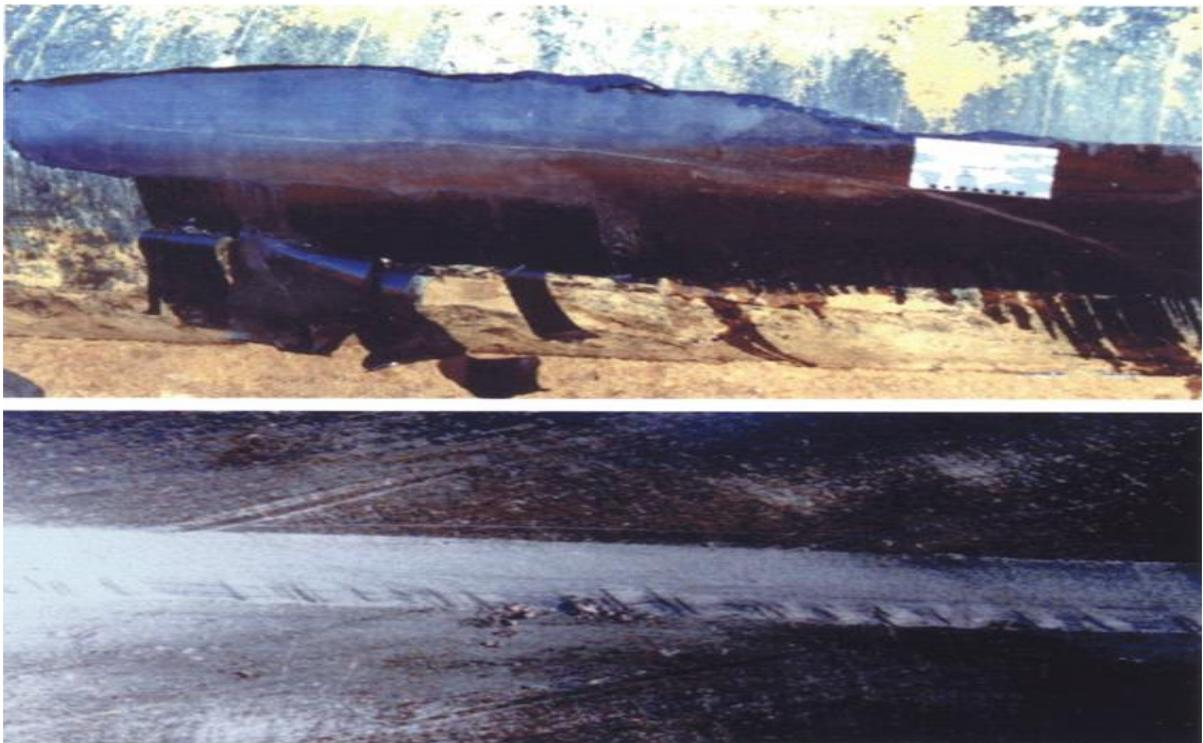
Figure 9. *Dents, depth 3 mm*
