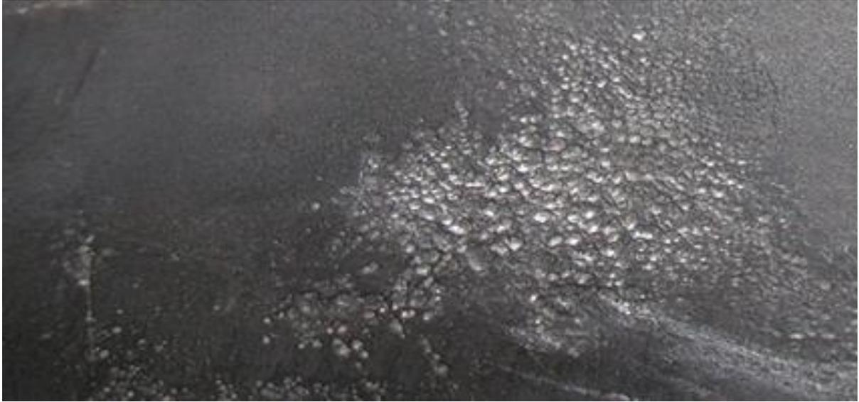
Figure 4. *Pitting corrosion, with depth up to 5 mm, on external pipe surface*
