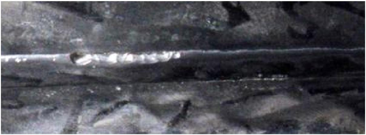
Figure 7. *Stress corrosion cracks with depth up to 8 mm, located along line of fusion of parent material and longitudinal weld (factory made)*
