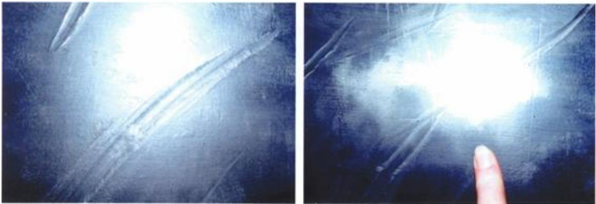
Figure 8. *Dents, depth 3 mm*
