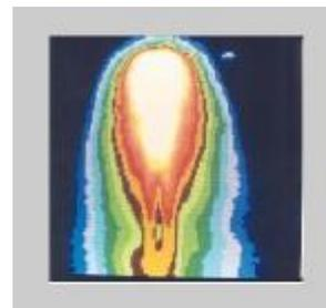
Figure 6: Thermograph of weld with air gap
