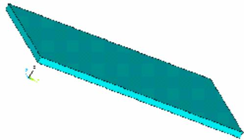
Figure 9: FEM model of 7 mm thick steel plate
