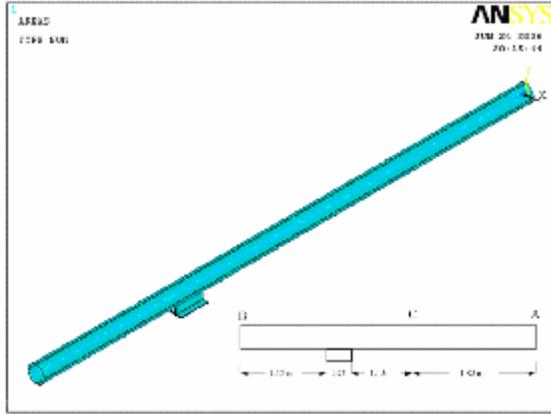
Figure 2: FEM model of pipe with welded support only
