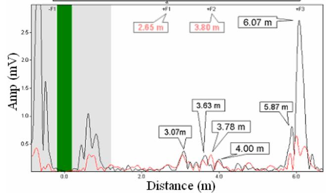
Figure 14: 32 kHz experimental result of a pipe with support and a defect
