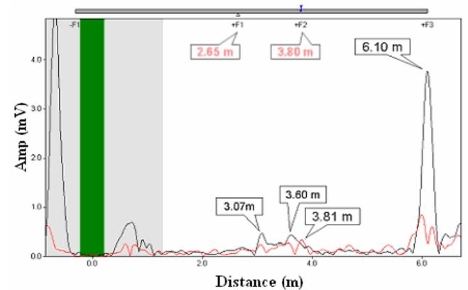
Figure 15: 28 kHz experimental result of a pipe with support and a defect
