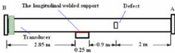
Figure 12: The diagram of the experiment setup
