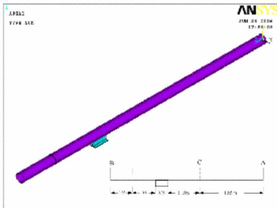
Figure 3: FEM model of pipe with welded support and defect
