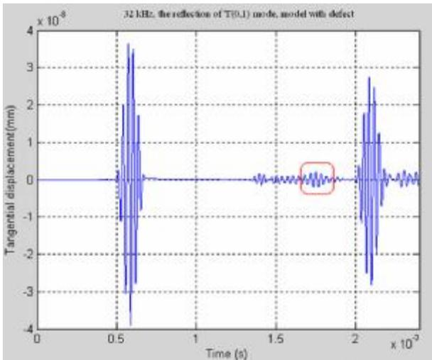
Figure 7: The time history of  $T(0,1)$  mode at monitored line C, defect model
