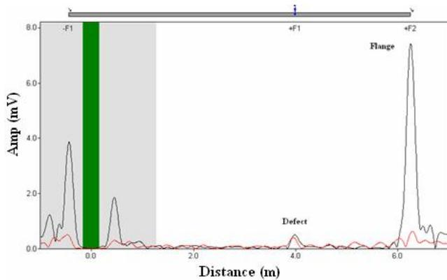
Figure 16: 28 kHz experimental result of a pipe with a defect only
