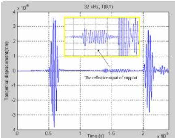
Figure 5: The time history of  $T(0,1)$  mode at monitored line C
