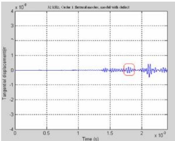
Figure 8: The time history of order 1 flexural modes at monitored line C, defect model
