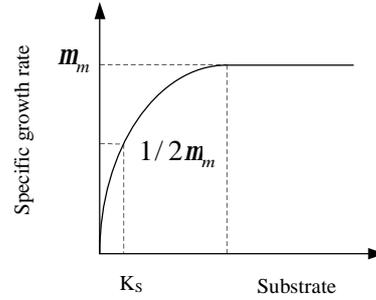
Figure 1. Growth curve following monod's equation
