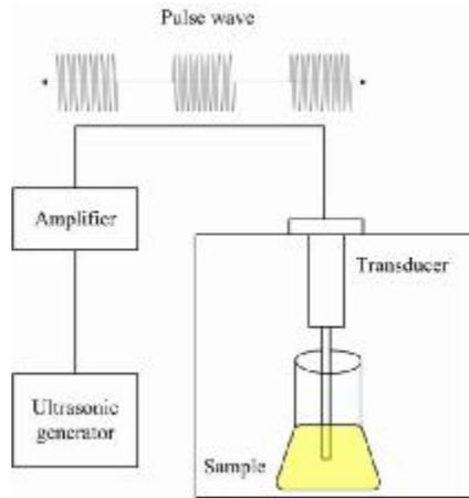
Figure 2. System of ultrasonic stimulation
