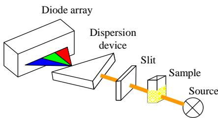
Figure 3. Optical density measuring technique
