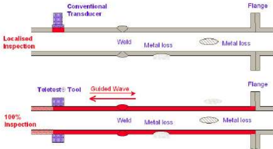
Figure 3: Principle of long range testing compared with conventional ultrasonic
