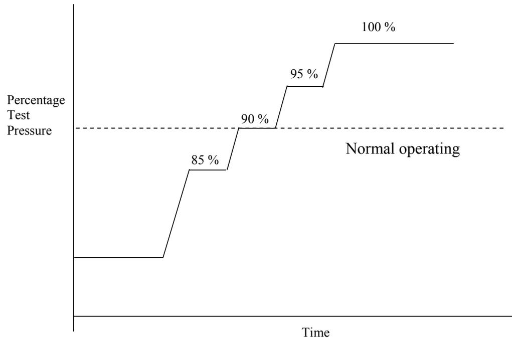
**Figure 9** Pressurisation program, all hold periods are 10 minutes except for last which is 30 minutes.
