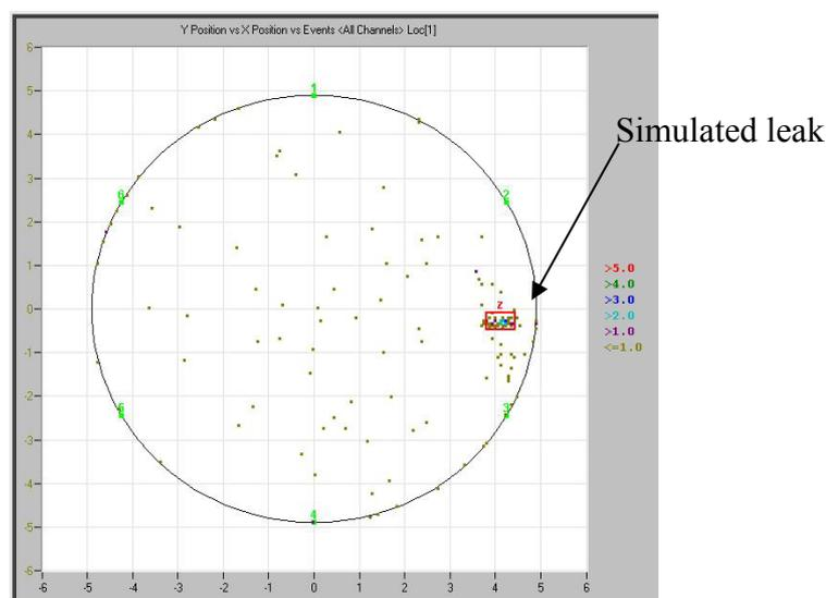
**Figure 13** Location of a simulated leak in a storage tank.
