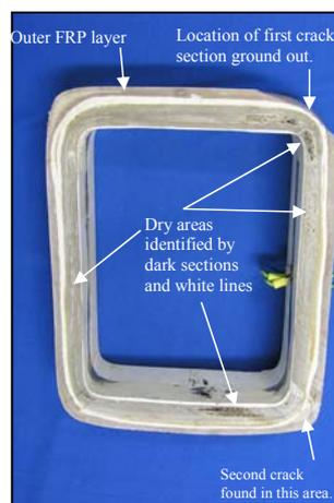
**Figure 7** Defects undetectable via conventional NDT
