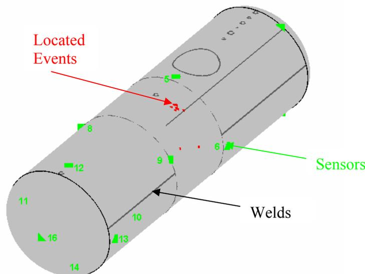
**Figure 8** Drawing of vessel to be tested, green squares indicate sensors position, weld seams and pipe fittings are also drawn. Red dots are simulated events located on surface.
