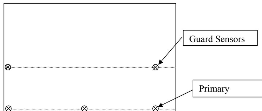
**Figure 12** Sensor layout on above ground storage tank. (Side elevation)
