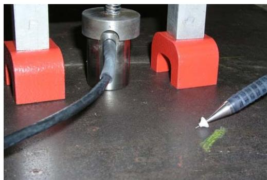
**Figure 5** Sensor mounted on steel vessel during calibration.
