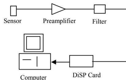
**Figure 3** Typical single channel AE system
