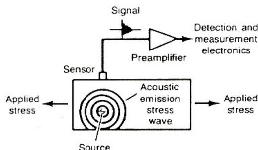
**Figure 1** Generation and detection of AE from an active source under stress[4].
