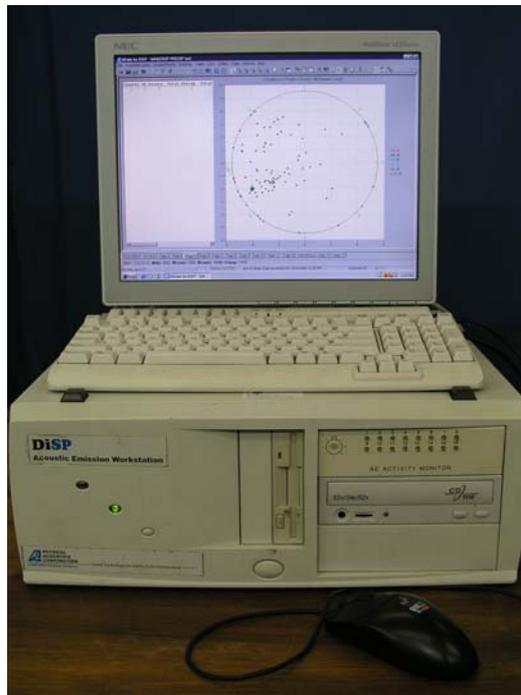
**Figure 4** PAC DiSP AE monitoring system showing AST bottom location results.
