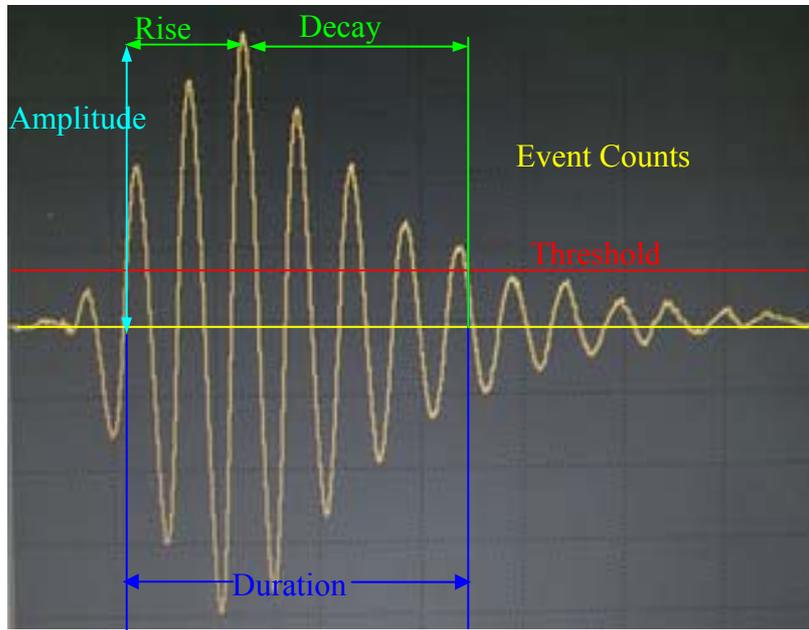
**Figure 2** Characteristics of the AE pulse.
