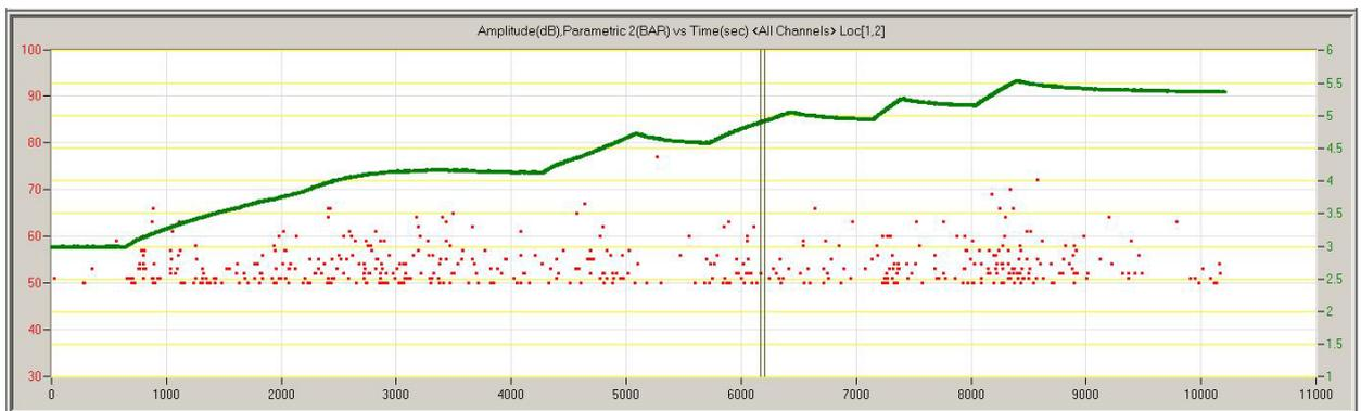
**Figure 10** Test results for vessel, green line is pressure in vessel while red dots indicated AE activity versus time.
