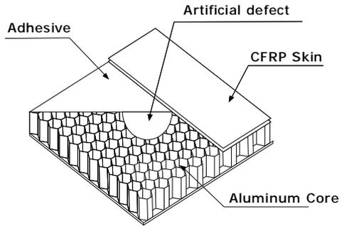
(a) Artificial delamination defect-specimen A
