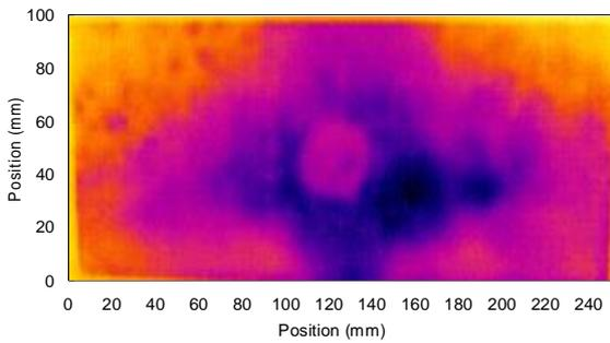
(a) Thermal image of artificial delamination defect
