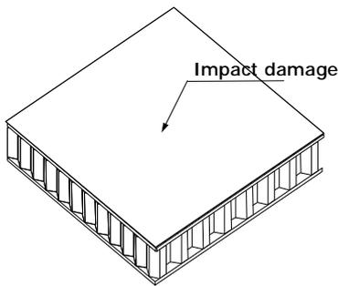
(b) Impact-induced delamination defect-specimen B
