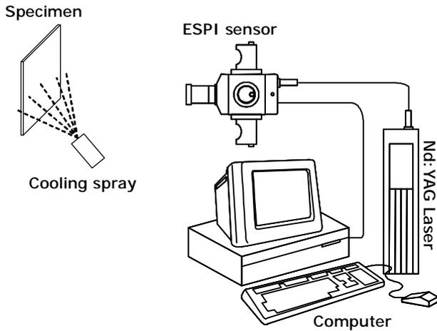
Figure 1: *ESPI measures the surface deformation under thermal loading and the difference of thermal expansion coefficient between sound part and defect part indicates the defect size and location.*
