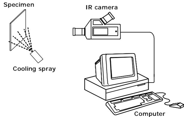
Figure 2: *Thermal loading gives temperature change due to thermal conductivity. If temperature difference between sound part and defect is large enough, the defect size and location can be recognized by 2 dimensional thermal image.*
