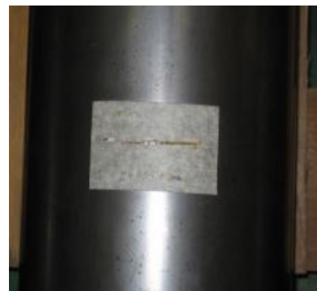
Figure 9 : photos of artificial notche in city gas pipe.
