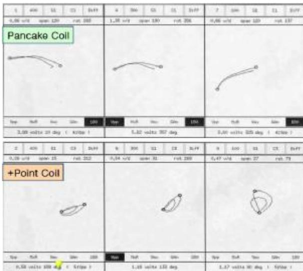
Figure 17: Phase Rotation of Volumetric Type Titanium with Sludge
