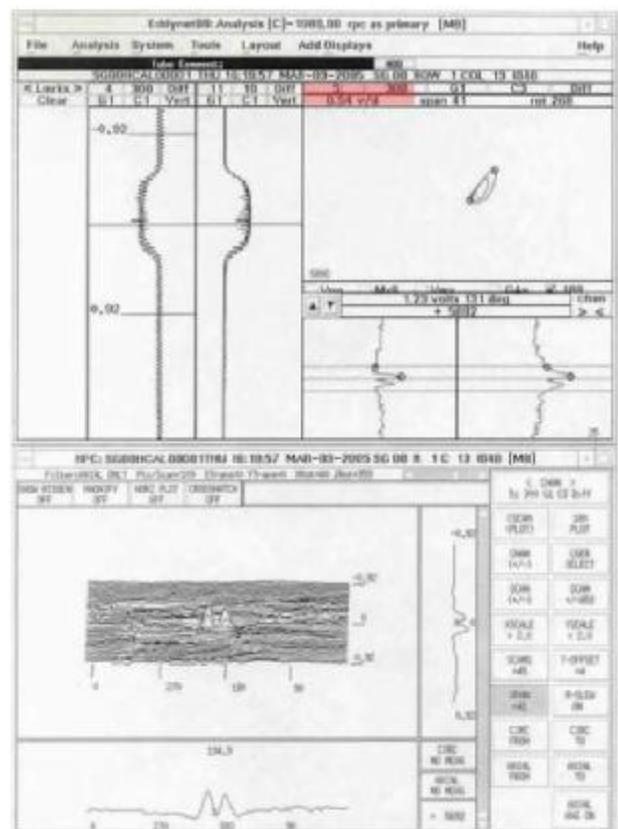
Figure 16: Volumetric Type Titanium Response with Sludge (+Point)
