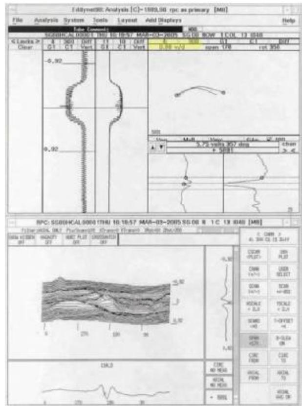
Figure 15: Volumetric Type Titanium Response with Sludge (Pancake)
