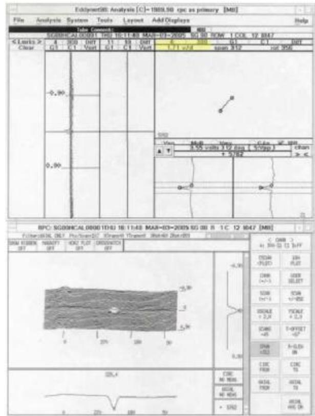
Figure 12: Volumetric Type Titanium Response (Pancake)
