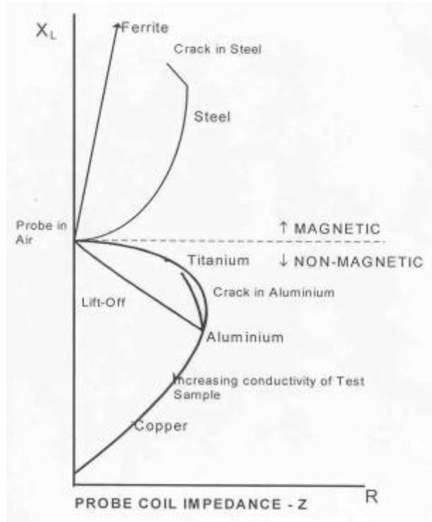
Figure 2: Conductivity of Various Materials
