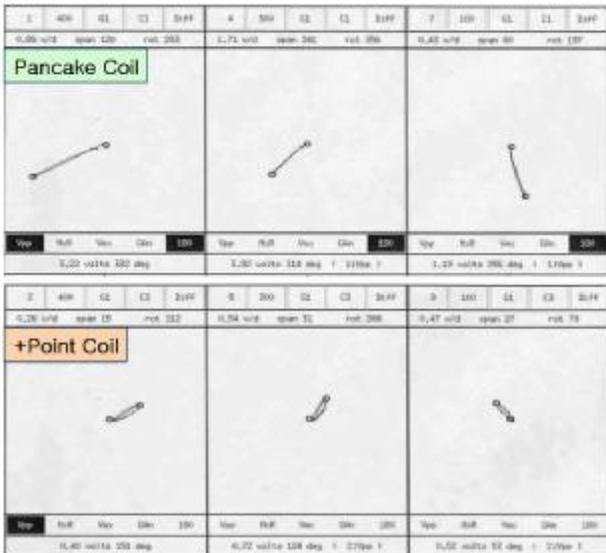
Figure 14: Phase Rotation of Volumetric Type Titanium
