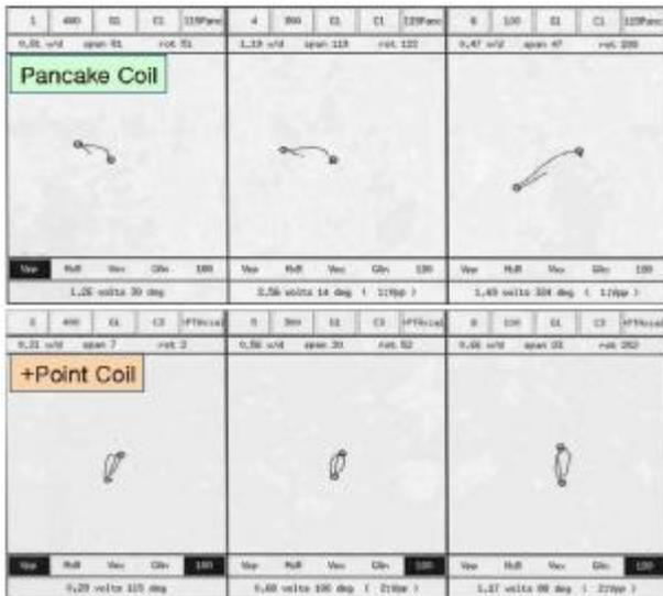
Figure 7: Phase Rotation of VOL-like Indication
