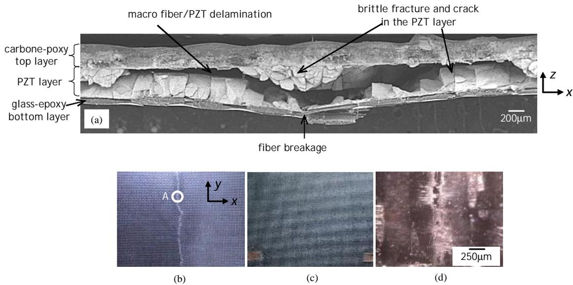
Figure 8: *Fractography* : (a) various fracture mechanisms of the PCA-A, (b) the main cracking on the surface of glass-epoxy bottom layer; (c) no damage in the carbon-epoxy top layer; (d) an enlarged view of circle A in photo (b).
