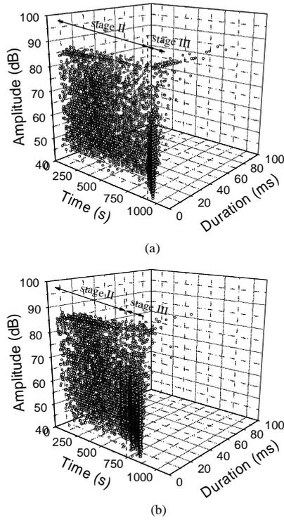
Figure 10: Distribution of the AE amplitude and duration versus the test time for (a) PCA-A and (b) PCA-B.
