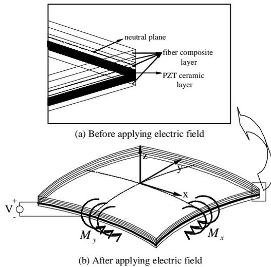
Figure 1: *The actuating principle of a stress biased piezoelectric composite actuator.*
