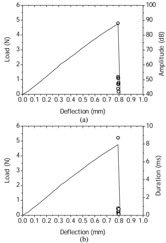
Figure 4: *AE signals from monolithic PZT ceramic: (a) a typical load-deflection curve and AE amplitude distribution; (b) a load-deflection curve and the distribution of duration.*
