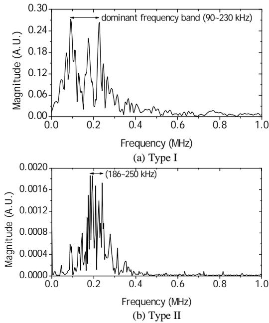
Figure 5: Typical FFT results of an AE signal from PZT ceramic: (a) at  $P_{max}$  and (b) after  $P_{max}$ .
