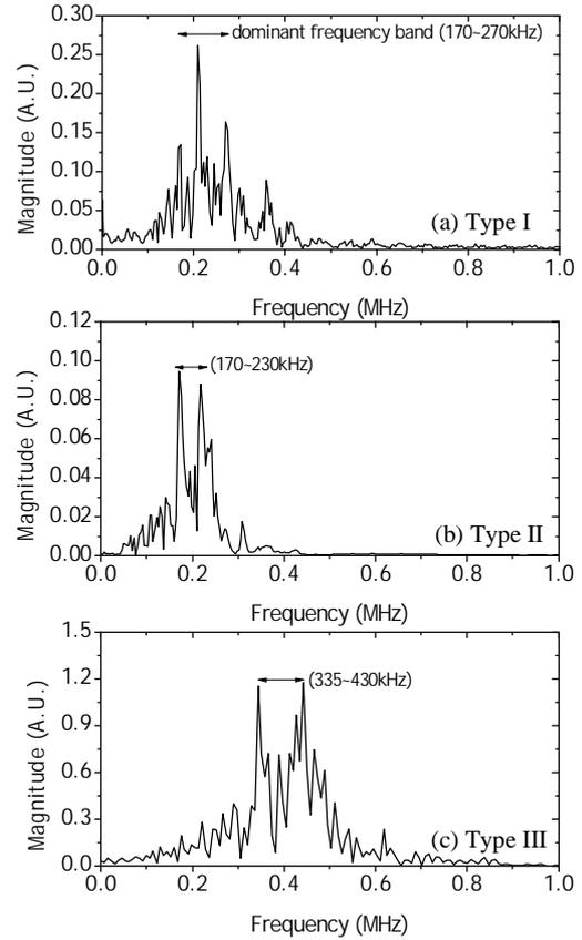
Figure 11: FFT results for representative AE signals according to the fracture process: (a) a low dominant frequency band with a high magnitude, (b) a low dominant frequency band with a low magnitude and (c) a high dominant frequency band with a high magnitude.
