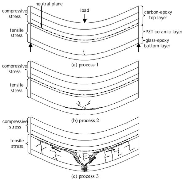
Figure 12: The bending fracture process of crack propagation and delamination growth in the PCA-A subjected to a bending load.
