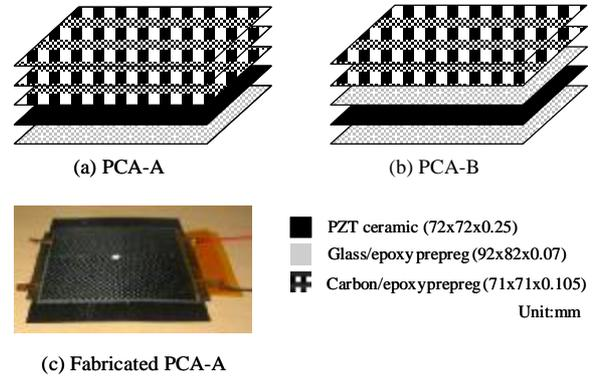
Figure 2: *Lay-up configuration of (a) the PCA-A and (b) the PCA-B; (c) a photograph of the fabricated PCA-A.*
