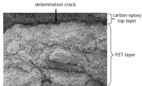
Figure 7: Scanning electron micrograph of the fractured surface in PCA-A: delamination between the fiber-PZT interface layers and brittle fracture and cracks in the PZT layer
