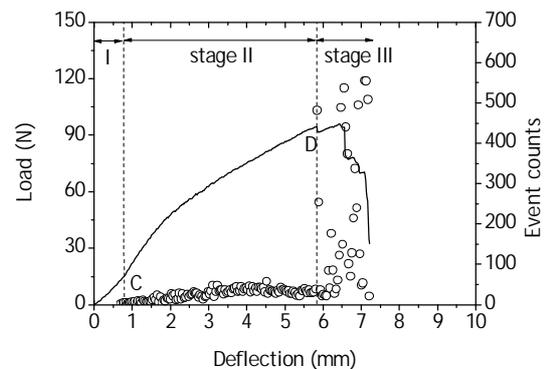
Figure 9: A load-deflection curve and the corresponding behavior of AE counts for the PCA-B under a bending load.
