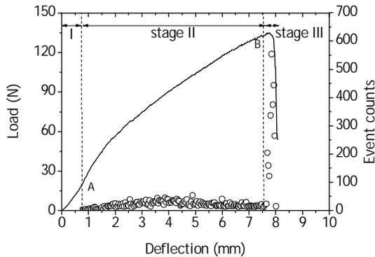
Figure 6: A load-deflection curve and the corresponding behavior of AE counts for the PCA-A under a bending load.
