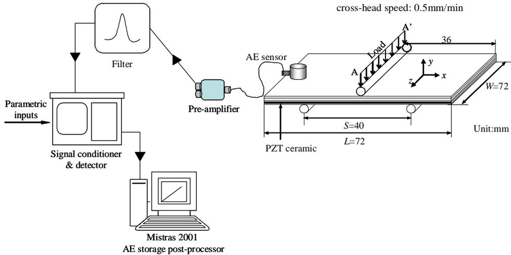
Figure 3: *Experimental set-up for a three-point bending test and an AE data acquisition.*
