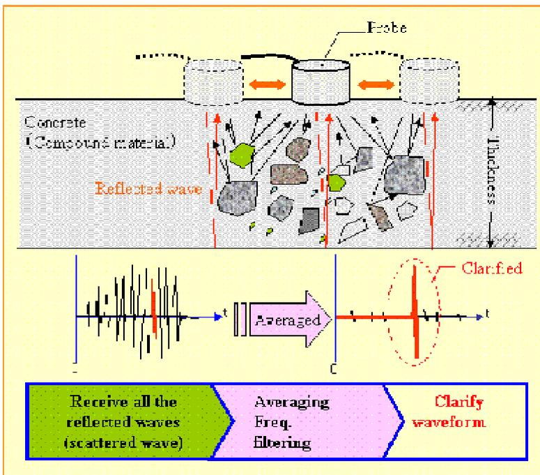
Fig.6 Concept of macroscopic ultrasonic inspection technology
