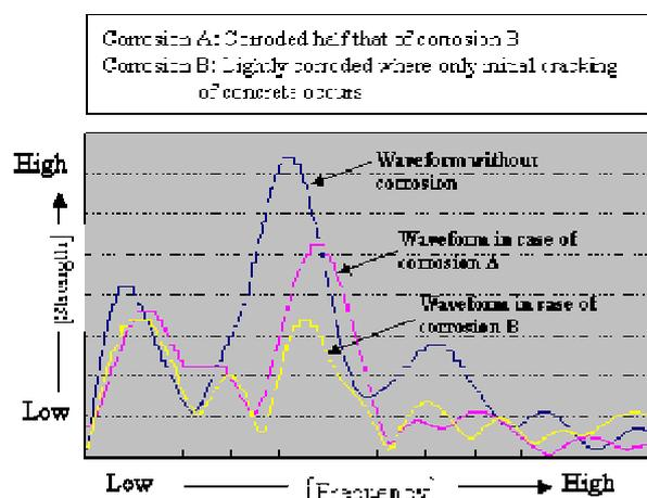
Fig.11 Frequency spectrum of wave reflected from reinforcement
