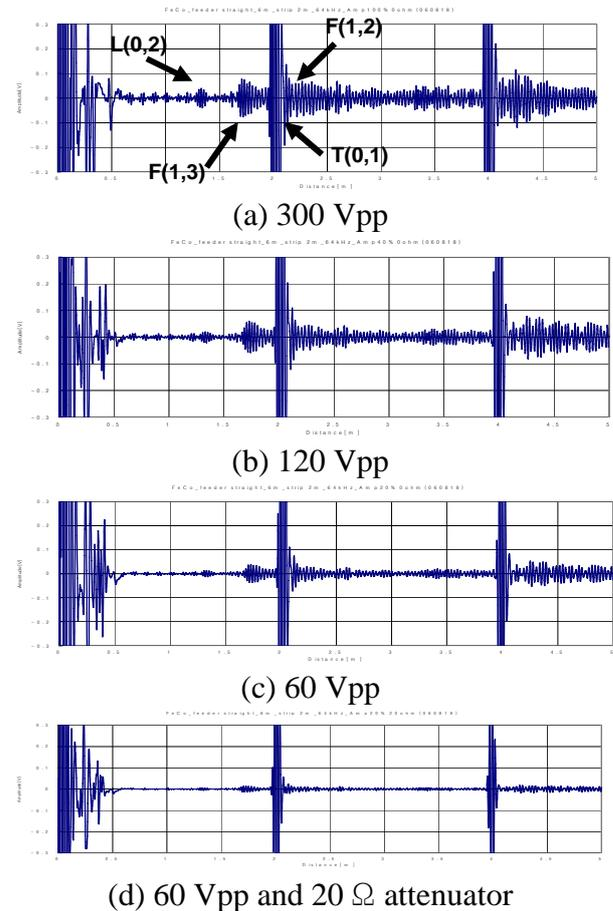
Fig. 4 Effect of alternating voltage.
