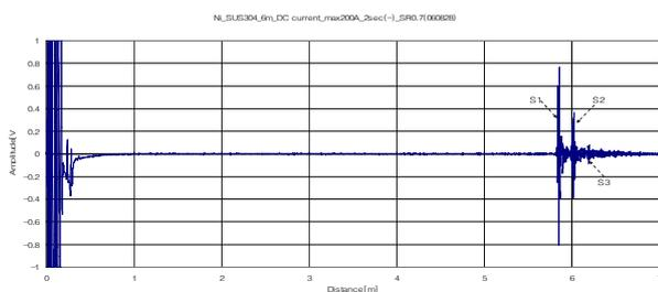
Fig. 6 Signals from the stainless steel tube by a circumferentially bias magnetized Ni strip.
