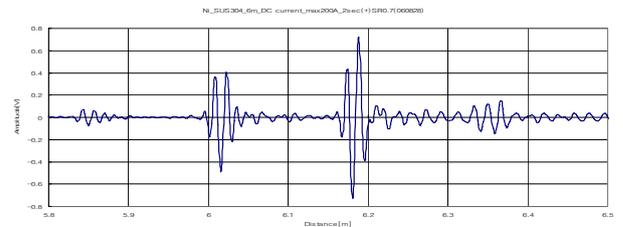
Fig. 8 Enlarged signal shape from different reflection of the tube end.
