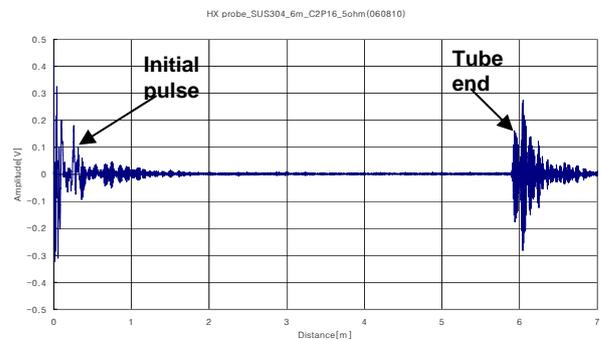
Fig. 9 Signal from stainless steel 304 heat exchanger tube using in-bore torsional guided wave probe.
