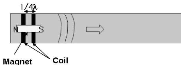
Fig. 3 A schematic design for a longitudinal vibration mode with a magnetostrictive transducer.
