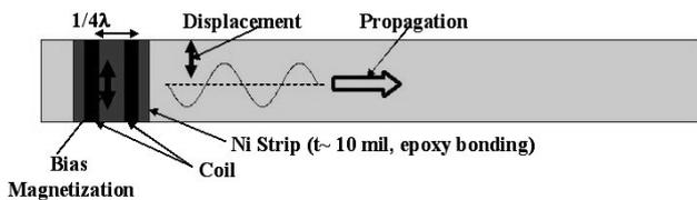
Fig. 2 A schematic design for the torsional vibration mode with a magnetostrictive transducer.
