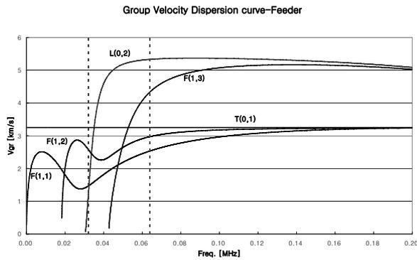
Fig. 5 Group velocity dispersion curve for a carbon steel pipe with an outer-diameter of 63.5 mm, a wall thickness of 6.5 mm.
