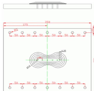
Figure 4: Geometry and dimension of the patched specimen
