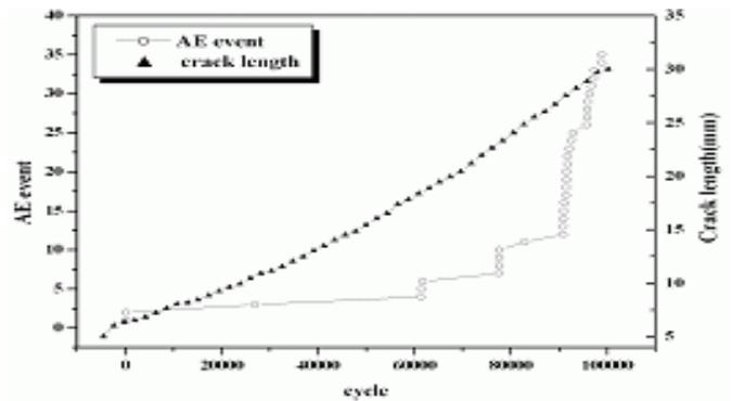
Figure 10: Cumulative AE events and the crack length vs. number of fatigue cycles
