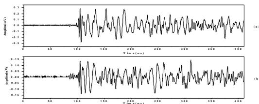
Figure 9: Effect of composite patch on the attenuation of simulated AE signals by pencil-lead breaks
