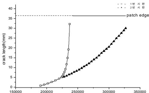
Figure 6: Growth behavior of the crack 10 in specimen #1 and specimen #2
