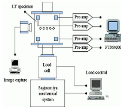
Figure 2: A schematic diagram of experimental setup
