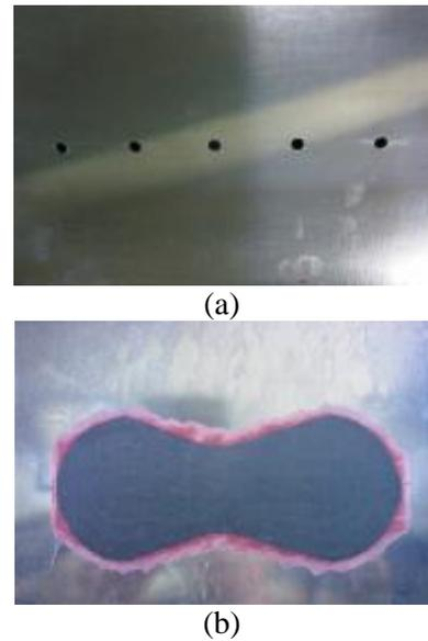
Figure 3: Photographs of the fatigue-cracked and the patch-repaired specimens; (a) before patching and (b) after patching
