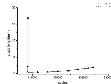
(d) Cracks No. 2 and No. 3 joined
