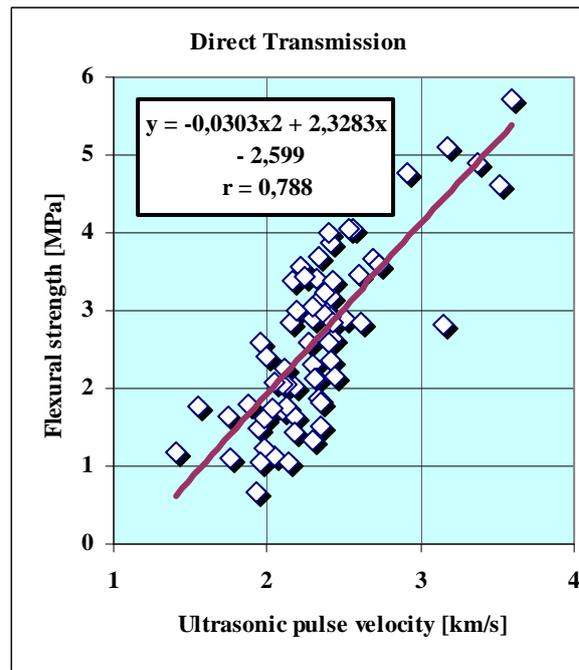
Figure 7b. Relation between flexural strength and ultrasonic pulse velocity
