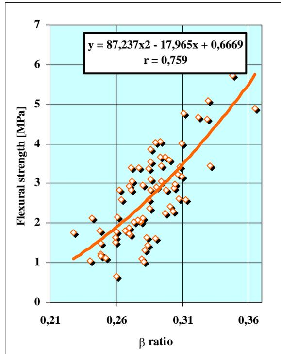
Figure 6b. Flexural strength from Waitzmann's scleroscope testing
