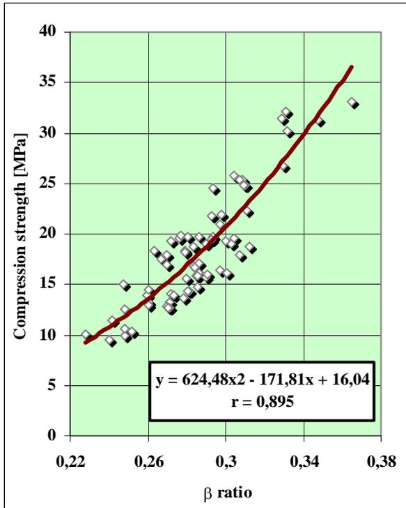
Figure 6a. Compression strength from Waitzmann's scleroscope testing
