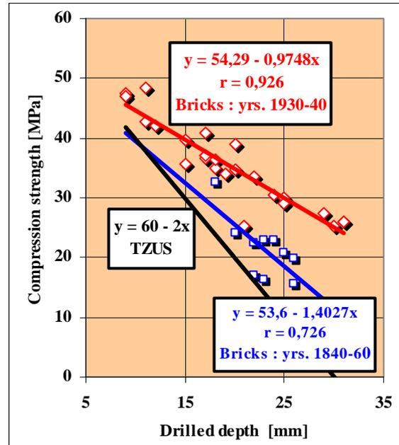
Figure 10. Comparison of strength measurement results by TZUS drill
