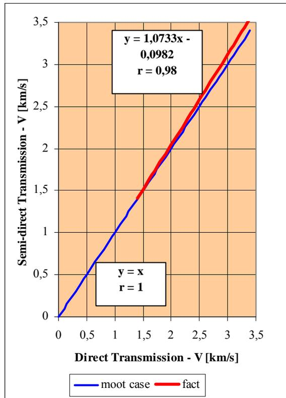
Figure 8b. Comparison between theoretical and actual V relations for different ways of transmission
