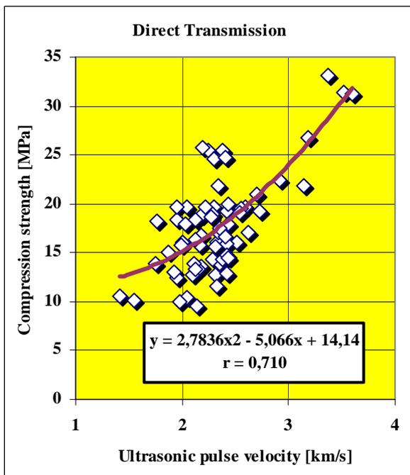
Figure 7a. Relation between compression strength and ultrasonic pulse velocity
