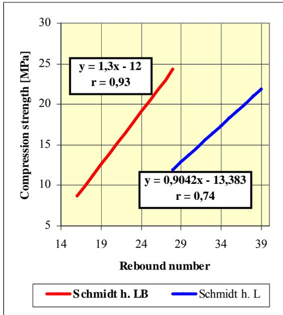
Figure 9. Comparison of measurement results by Schmidt impact hammer types LB and L
