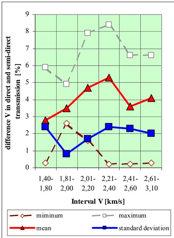
Figure 8a. Comparison of differences V for different ways of transmission
