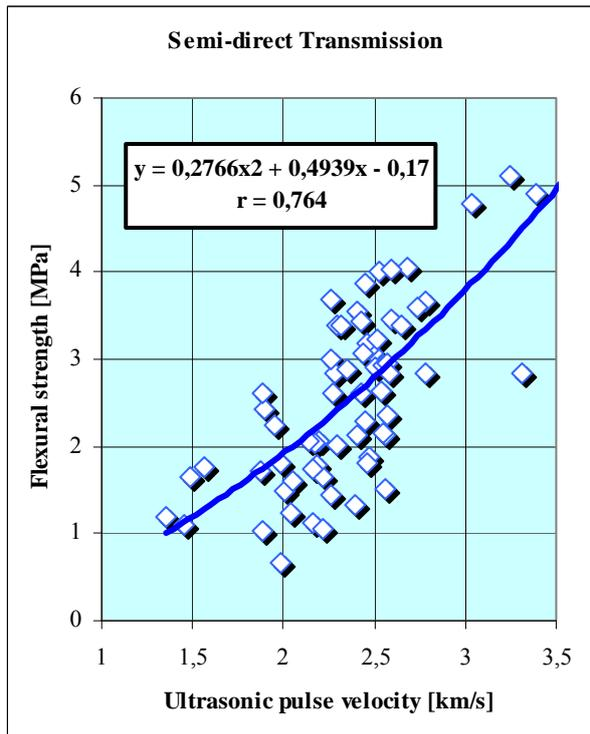
Figure 7d. Relation between flexural strength and ultrasonic pulse velocity
