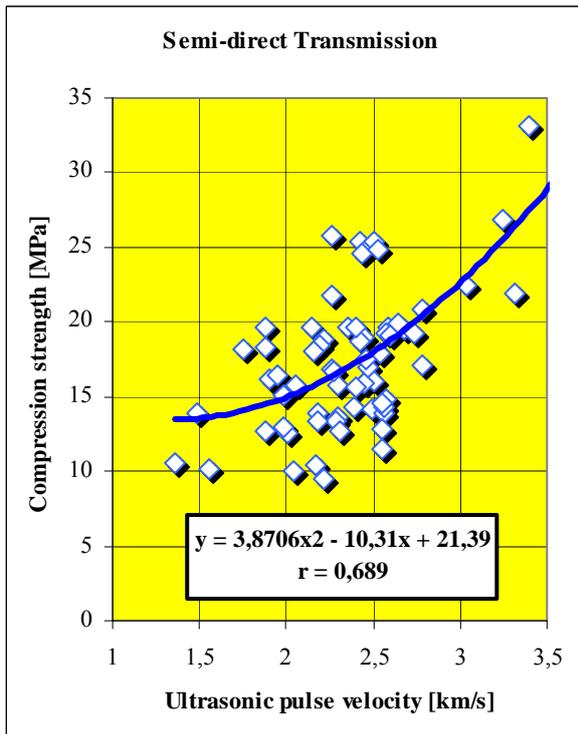
Figure 7c. Relation between compression strength and ultrasonic pulse velocity
