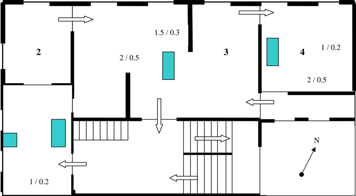
Fig. 6. Daylight Factor without and with solar protection film on the windows
