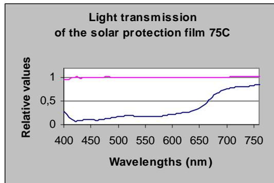
Fig. 4. Light transmission curve of the SS75C
