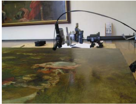
Figure 2. Colour measurement on site
