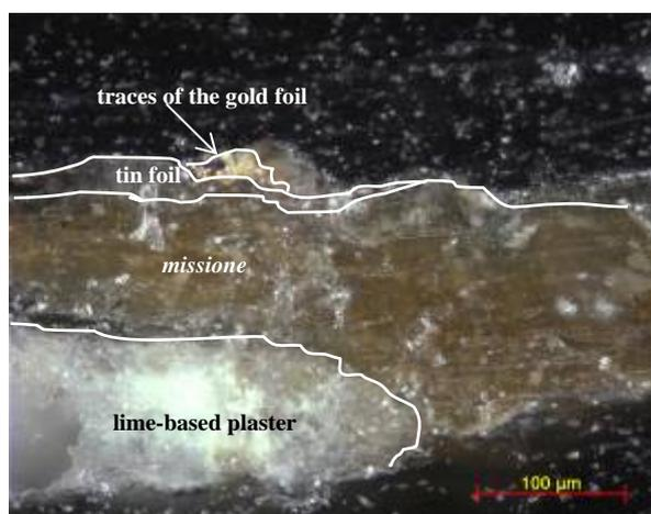
Fig. 3. Stratigraphy of the halo (cross section, incident light).
