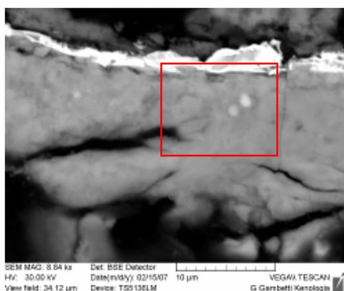
Fig. 6. BSE image of the metal foils.
