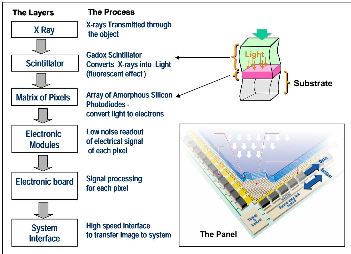
Figure 1: Amorphous Silicone Flat Panel Structure
