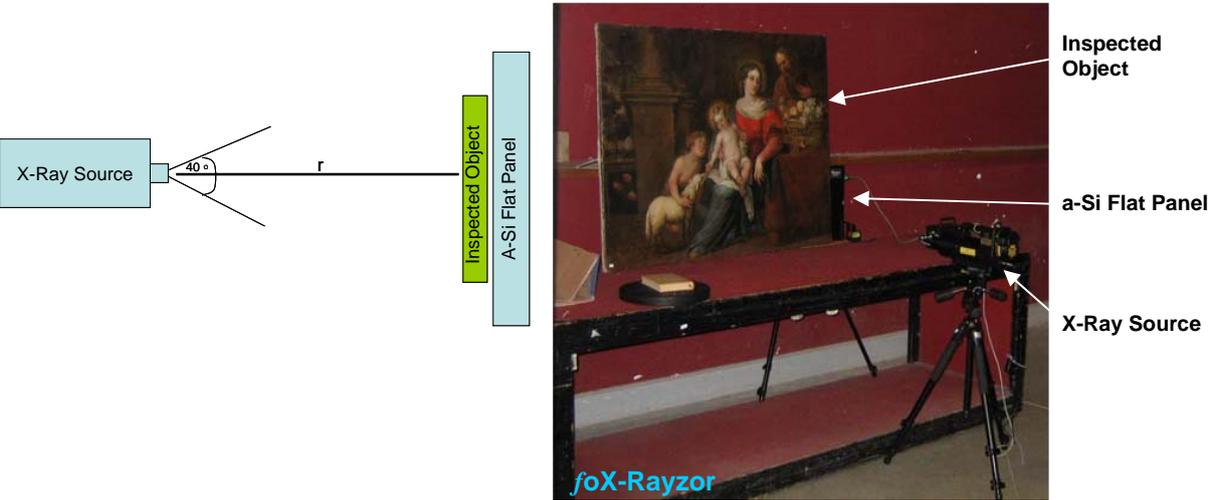
Figure 9: Setup for DR Inspection
