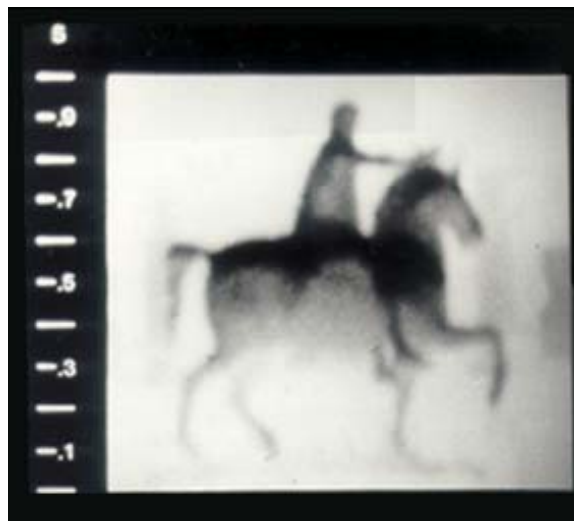
Fig. 4 - Thermogram of the equestrian monument recorded in the environmental thermal decrease phase
