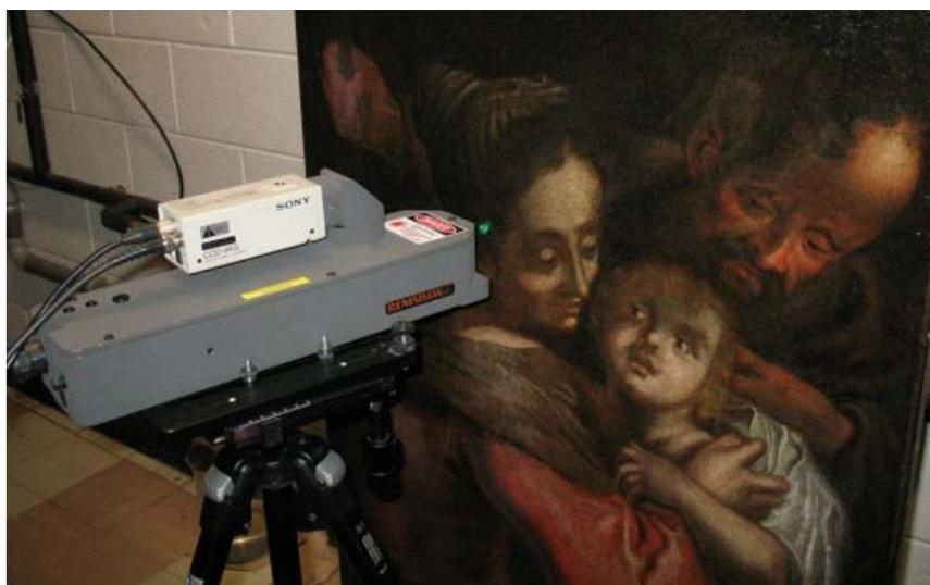
*Fig.8 Renishaw® Fiber optic Raman analyzer in operation.
