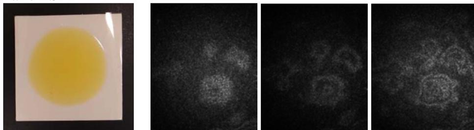
Figure 7: *a. Image of Liquol pour and ESPI fringes of gas release after the pour at b.  $\Delta t = 965$ mins c.  $\Delta t = 980$ mins d.  $\Delta t = 995$ mins*
