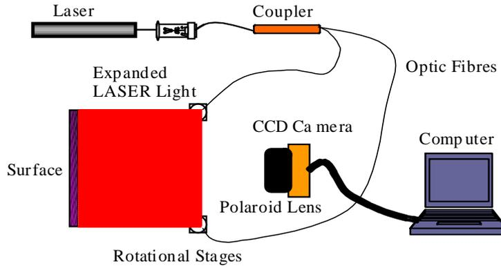
Figure 1: Experimental set-up for In-Plane ESPI
