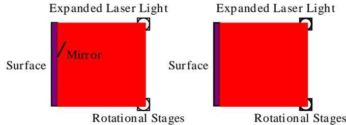
Figure 2: Beam alignment for (a) Out-of-Plane ESPI (b) LSCI
