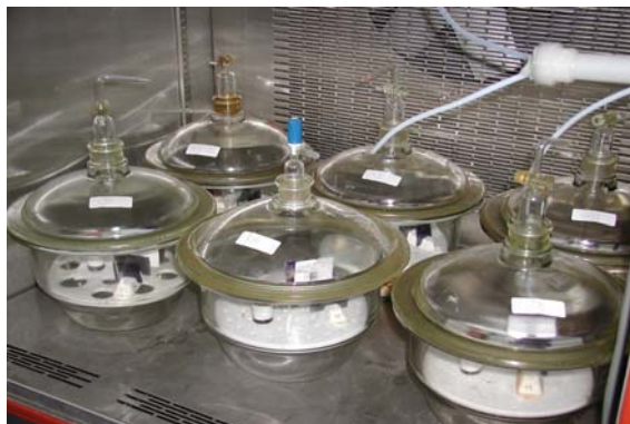
Fig. 2: Desiccators with organic acids and glass samples inside the climate chamber
