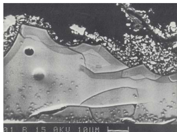
Fig. 11: Electron microscope picture of the cross section through an enamel fragment of an object of art stored in a show case more than 20 years
