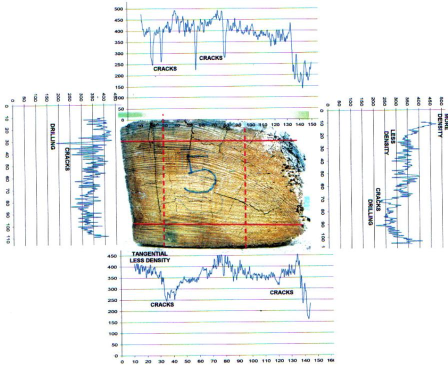
Fig. 2. Some of the microdrilling graphics obtained in probe 5
