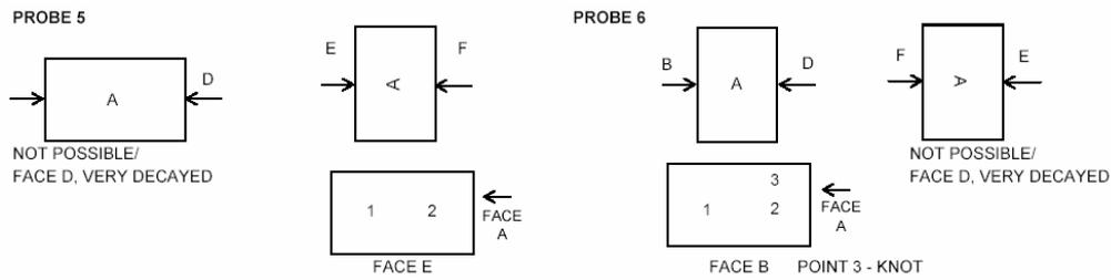
Fig. 4. Scheme of ultrasonic testing in probes 5 and 6
