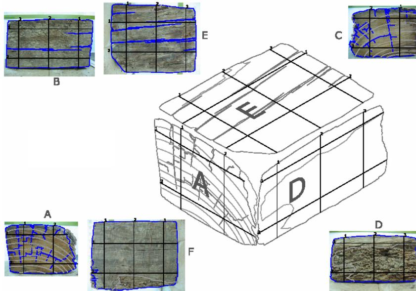
Fig. 1. Drawing of the probes, in this case Probe 5, showing grid for microdrilling
