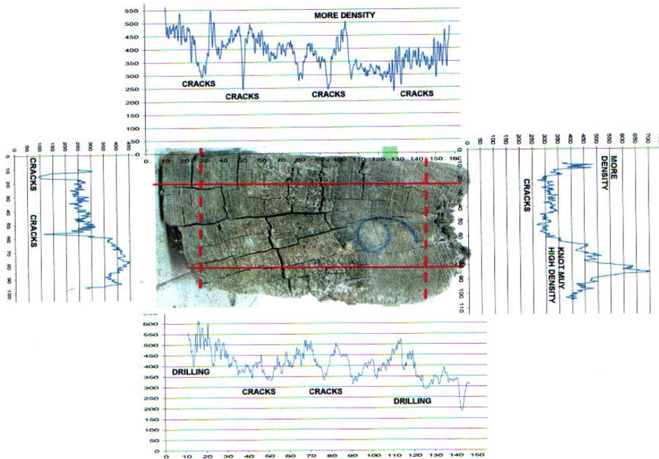
Fig. 3. Some of the microdrilling graphics obtained in probe 6
