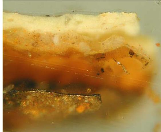
Figure 13. Cross section showing the original gold lamina (lower part of the picture) covered by a first silver lamina, turned into brown, and a second very recent gold lamina on the top.
