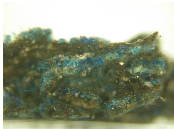
Figure 11. Cross section from the dentil of the superior freeze of the frame. Azurite pigment embedded in organic medium turned into brown.
