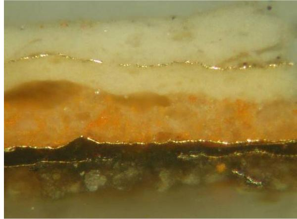
Figure 17. Cross section showing the sequence of three gold laminae and a silver lamina (turned into black silver sulphide), in between the first and the second gold lamina.
