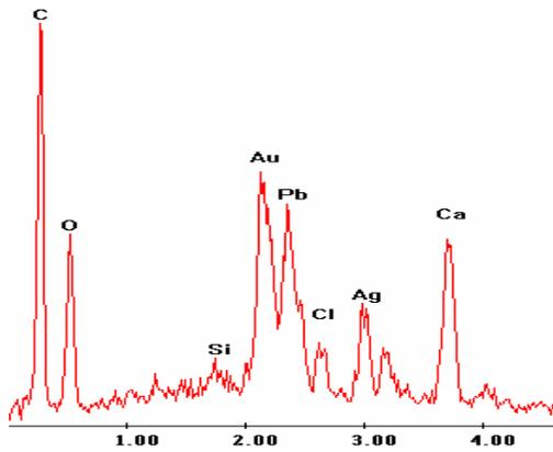
Figure 18. EDS microanalysis of the original gold lamina (layer **b**).
