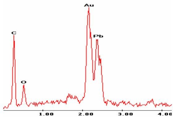
Figure 21. EDS microanalysis of the third gold lamina (layer **h**).
