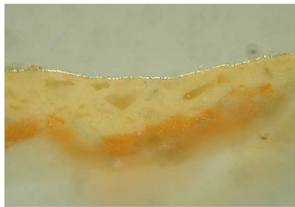
Figure 3. Cross section of the gilded layer from the basement of the column. The top gilded layer was applied on a white lead containing barite particles which are a marker of not original gold application.
