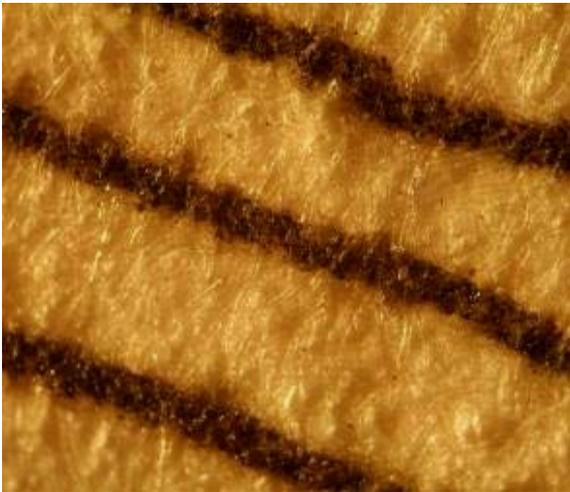
*Fig 9: macrophotograph from an original etching of "Museum Florentinum": ink permeates paper, each line is surrounded by tiny spots*
