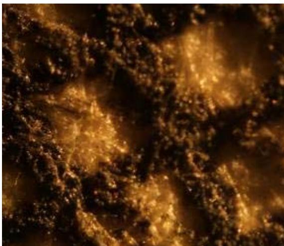
*Fig 5: macrophotograph from an original etching of "Museum Florentinum": the ink is raised on the paper and it is dull and granular*
