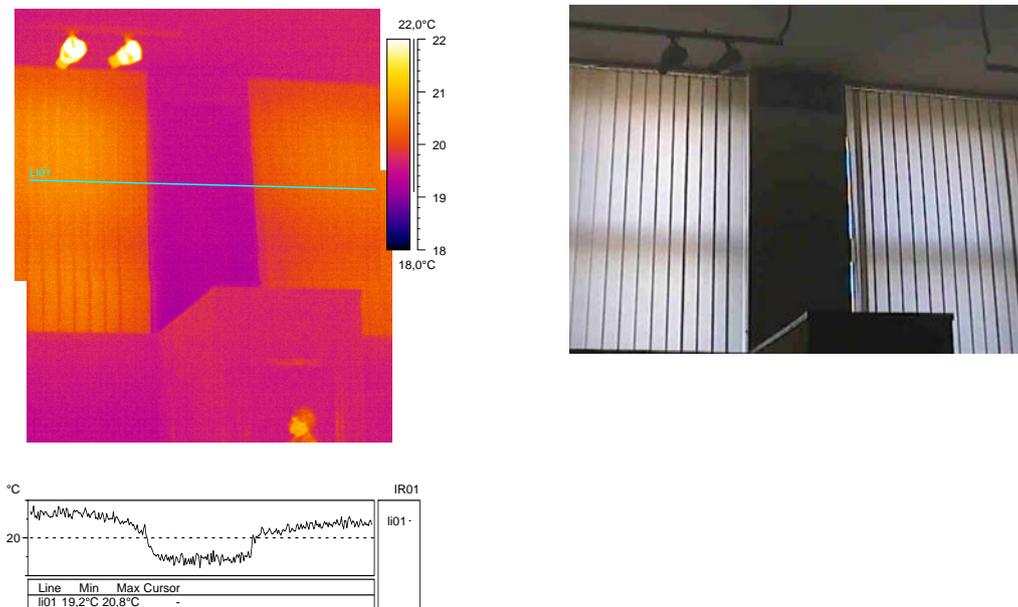
Fig.3. Temperature profile from the wall October noon
