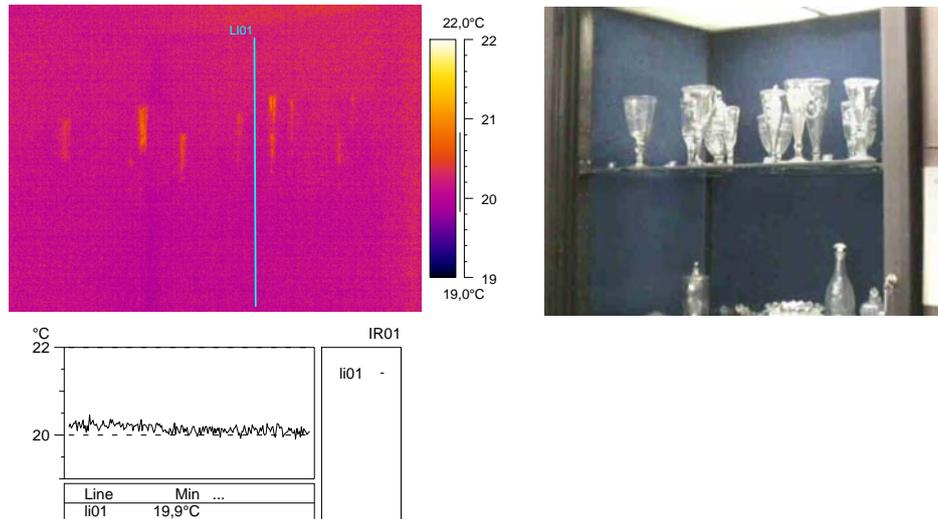
Fig.7. Temperature profile along chosen line in showcase F-9.
