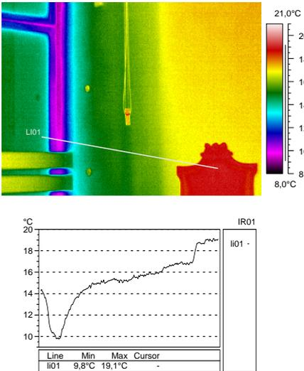
Fig.2 Termogram from room corner in hall nr 202 Januarz at. 11:16
