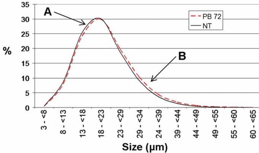
Fig. 1 - Wall thickness distribution of Lecce stone samples untreated (continuous line) and treated with PB 72 (broken line). The profiles were calculated on an average of 7 samples
