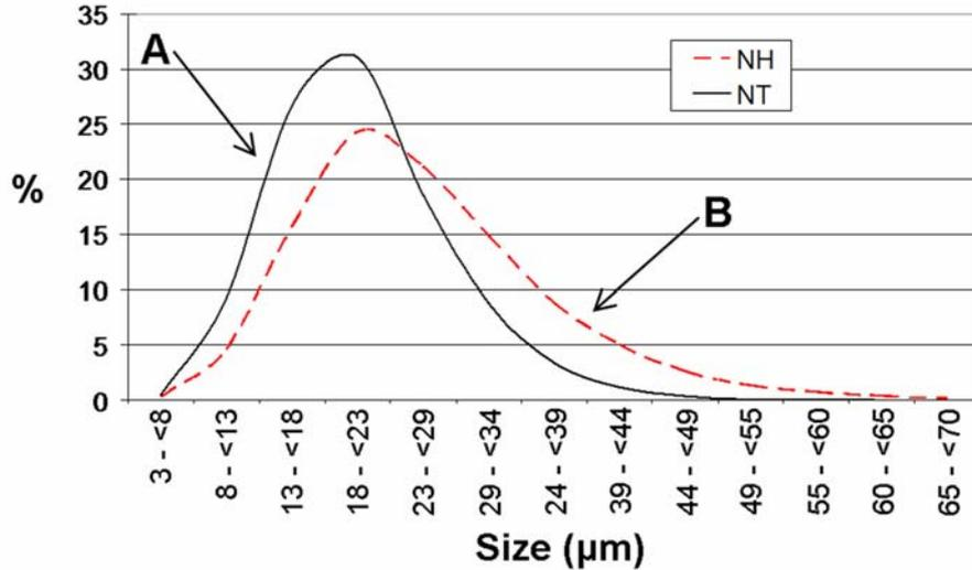
Fig. 2 – Wall thickness distribution of Set3 untreated (continuous line) and treated with NH (broken line). The profile shows the decrease of the thinner walls (A) and the increase of the thicker ones (B)
