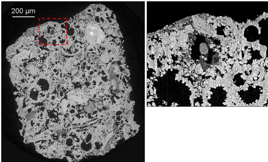
Fig. 3 – Cross section of Lecce stone treated with PB 72, obtained by means of SR-CT
