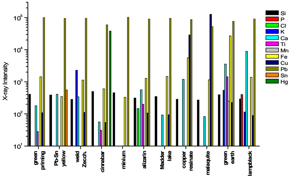
Figure 7. X-rays intensities detected for the pigments and lakes on the green priming (Table II).
