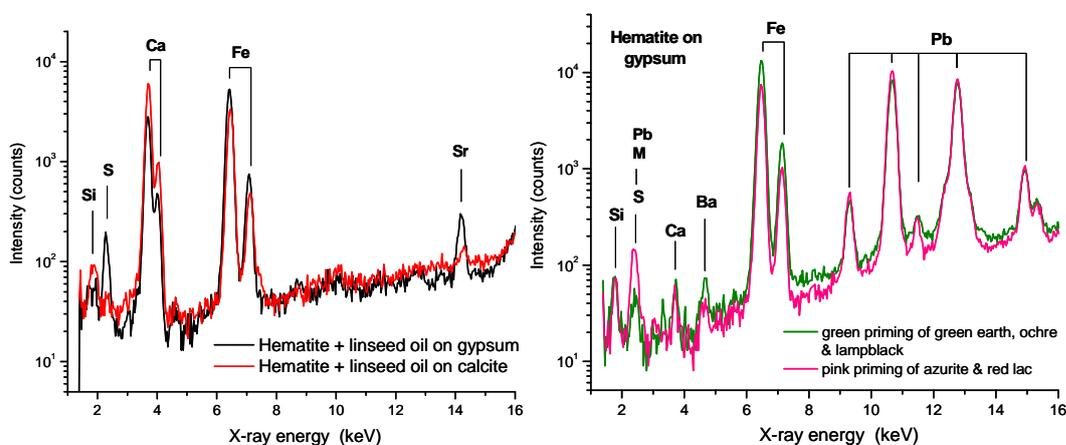
Figure 6. XRF spectra of hematite on gypsum and calcite grounds and various primings.
