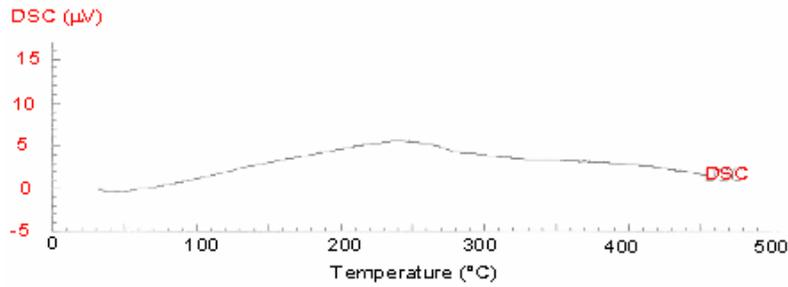
Fig. 6: DSC diagram: phase transformation at about 250°C is visible
