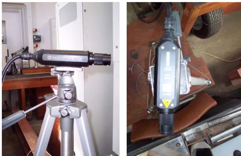
*Fig4 and Fig5 Compact Laser Vibrometer, CLV 700, Polytech*
