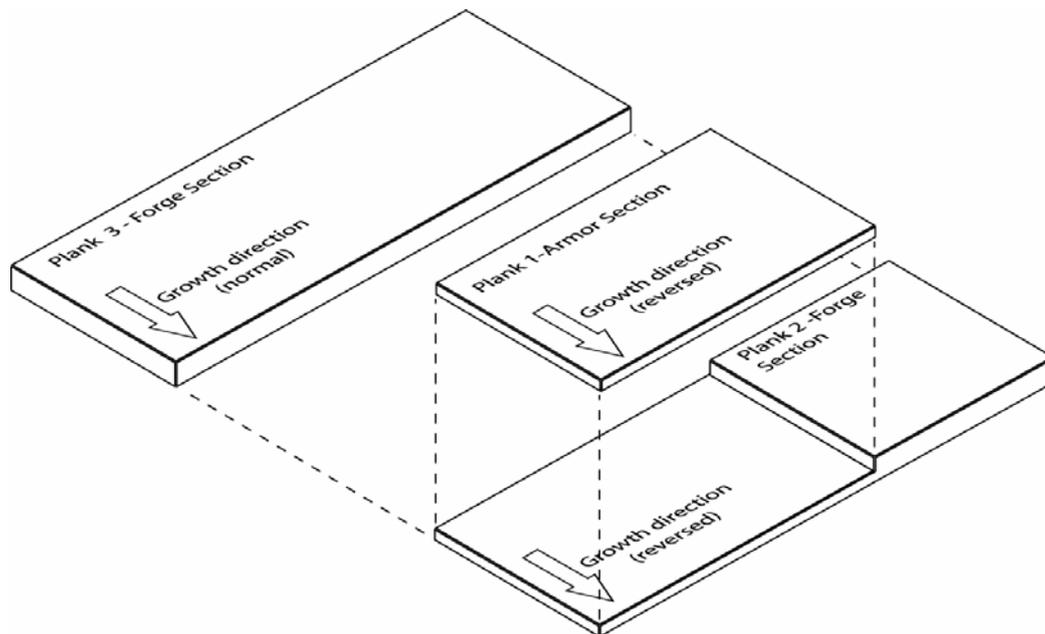
**Figure 2.** Construction of *The Armorer's Shop*, as revealed by optical microscopy and dendrochronology. Arrows indicate the growth direction of each of the wood planks. For the bottom two planks, this growth direction is reversed compared to conventional practice, in which planks are oriented so that their older, harder wood faces outward.
