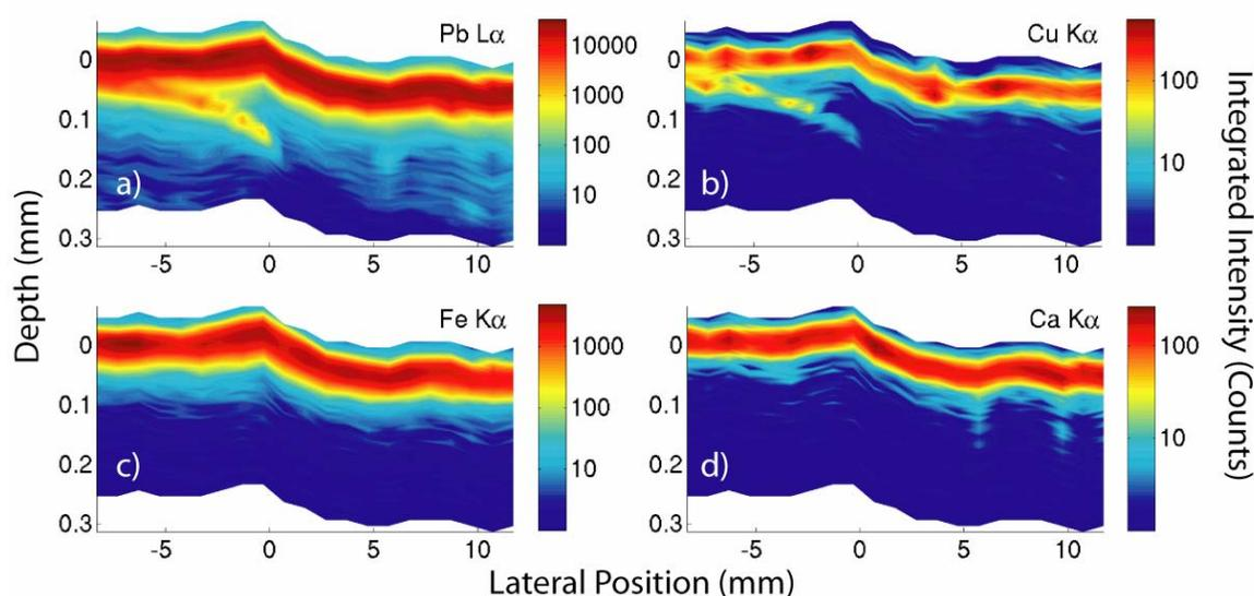
**Figure 4:** Virtual cross-section across the interface between parts 1 and 2, showing an earlier imprimatura on part 1. The position of the line scan is indicated in Fig. 1. (a), (b), and (d) show the fluorescence intensity on a logarithmic color scale. (c) shows the Cu K $\alpha$  concentration on a linear scale.
