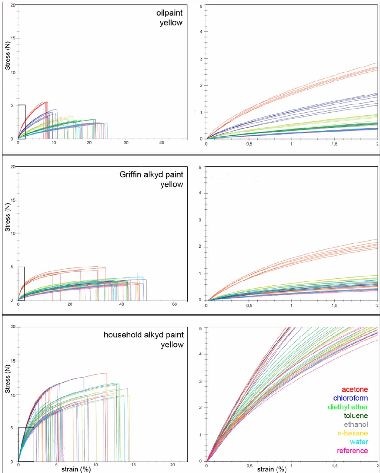
Fig. 9: Influence of solvent treatment on the mechanical film properties of the yellow oil paint (top), Griffin alkyd paint (centre) and DIY alkyd paint (below). Left: Total stress-strain diagram. Right: Detail of the elasticity modulus at 5N tensile force and 2 % elongation. Acetone causes the most marked embrittlement of the paint strips, followed by chloroform, diethylether, toluene and ethanol. *N*-hexane and water barely alter the mechanical properties at all.
