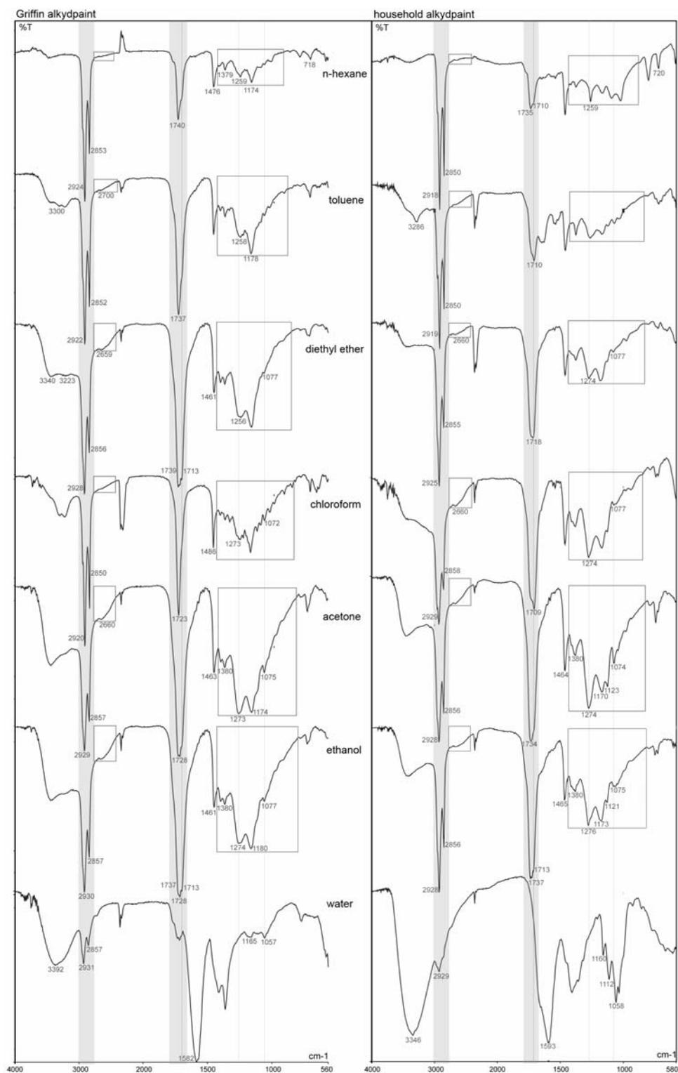
Fig. 6: Infrared spectra of the solvent extracts. The polarity of the solvents increases from top to bottom. Left: extracts from the white Griffin alkyd paint, right: extracts from the white DIY alkyd paint.
