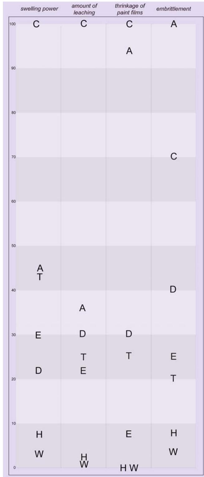
Fig. 10: Comparison of all the test results: They are not absolute figures but relative averages. The effect of the "strongest" solvent has been put at "100", and the effects of the other solvents rated accordingly lower. The embrittlement data were optically estimated on the basis of the determined elasticity moduli. (C = chloroform, A = acetone, T = toluene, E = ethanol, D = diethylether, H = hexane, W = water)
