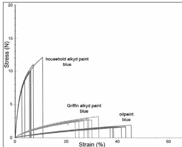
Fig. 7: Stress-strain diagram of the blue pigmented untreated DIY alkyd paints, Griffin alkyd paints and oil paints.
