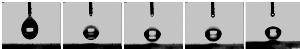
Figure 4: Water droplet bouncing on marble which was treated with siloxane and  $\text{SiO}_2$  nanoparticles
