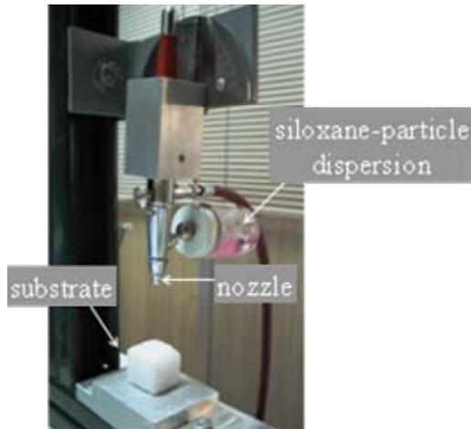
Figure 1. Spraying technique
