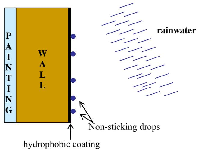
Figure 2. A protective coating applied on the outer surface of a monument must repel rainwater
