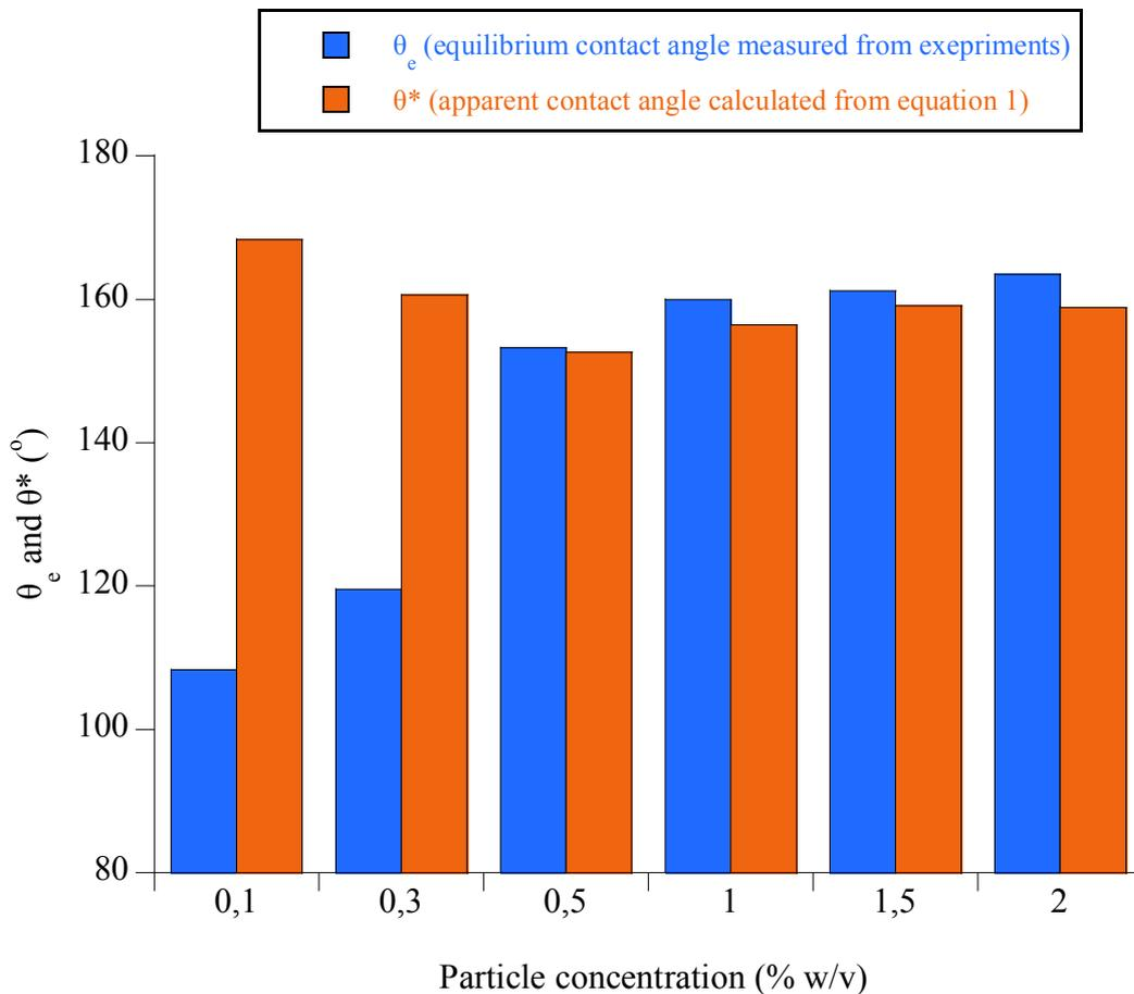
Figure 7. Equilibrium contact angle ( $\theta_e$ ) and apparent contact angle ( $\theta^*$ ) as a function of  $\phi_s$  for silonaxe-SiO<sub>2</sub> on glass.
