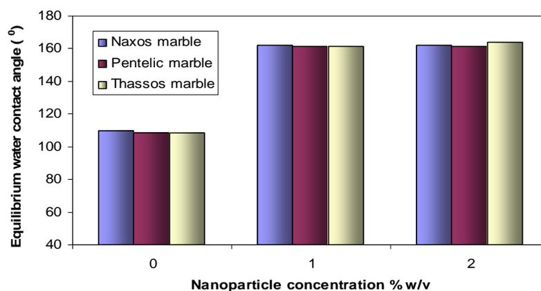
Figure 3: Equilibrium water contact angle ( $\theta_e$ ) as a function of particle concentration
