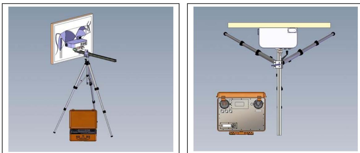
*Figure 1a and 1b. Two views of the positioning of the XRD/XRF in front of a painting.*
