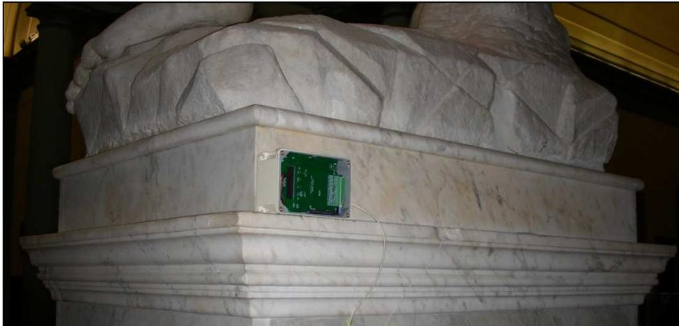
Figure 2 – The basement of David and the device Smartbrick
