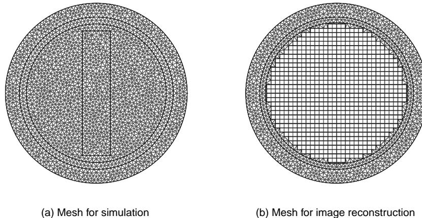
Figure 5: Examples of FEM meshes used in ECT
