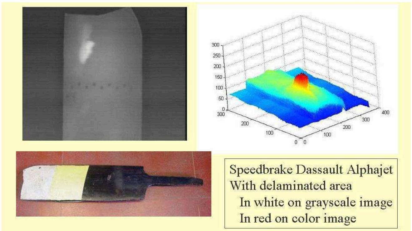
Figure 3 : Example of use of our military thermal imager to detect delamination on Belgian training Aircraft
