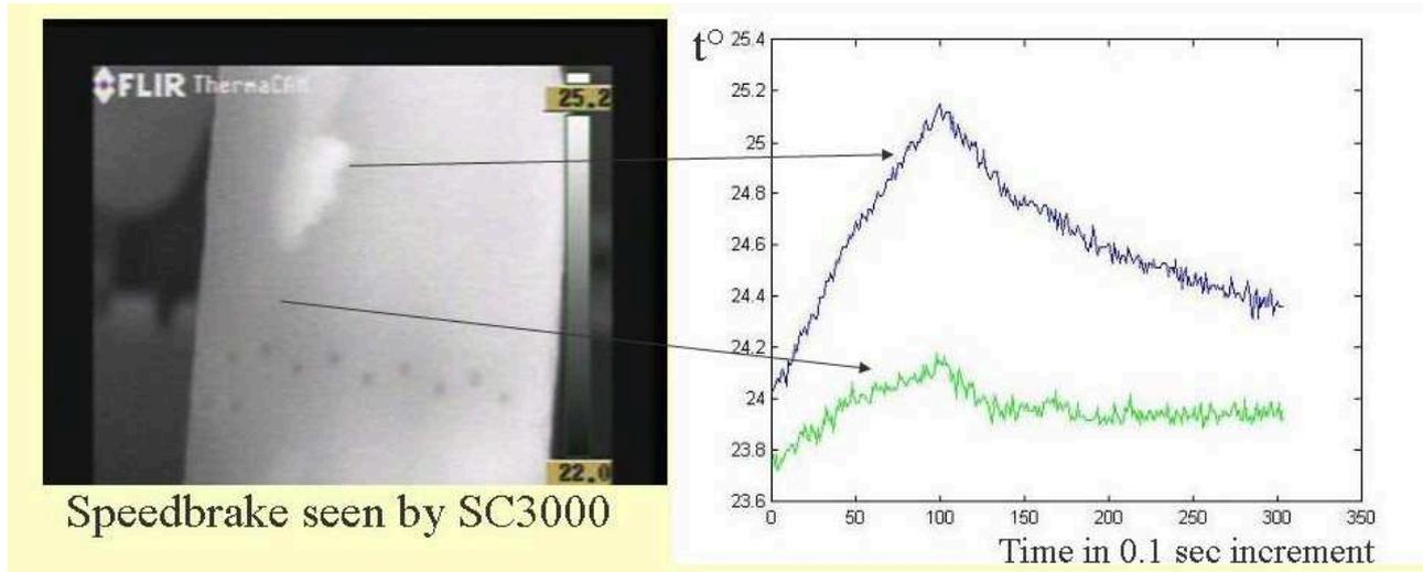
Figure 5 : Alphajet speedbrake tested with FLIR camera with T° evolution during 30 sec on 2 relevant points
