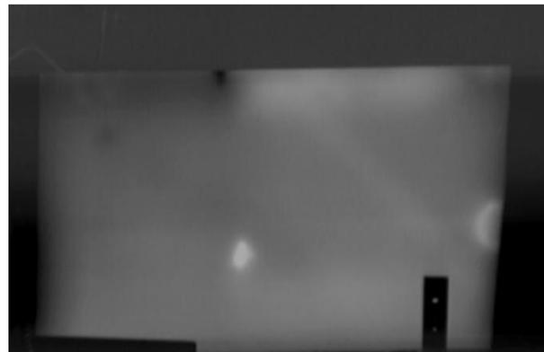
Figure 2 Left : composite part with hole type IQI,
