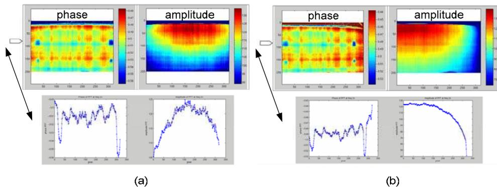
Fig. 3 Effect of orientation on phase and amplitude for *Specimen 1* made of CFRP with orientation of (a):  $0^\circ$  and (b):  $20^\circ$ . Second discrete frequency (0.167 Hz). Plots along image row are also shown.
