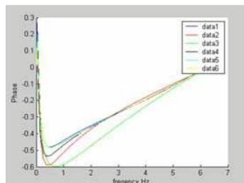
Fig. 5 Typical phase evolution from the shallowest to the deepest defect ranking (0.2 mm increment): 3, 2, 4, 5, 1 and data 6 is the selected reference area (non-defect). Results were obtained using 400 frames at an acquisition speed of 25 Hz, allowing a minimum frequency of 0.0625 Hz and maximum frequency of 12.5 Hz. Specimen orientation was 0°. *Specimen 1*.
