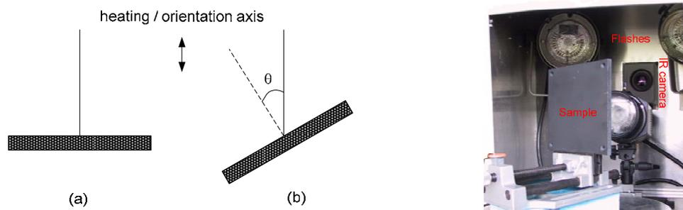
Figure 1 Flat and tilted plate (left), experimental set-up for IR thermography NDE (right).
