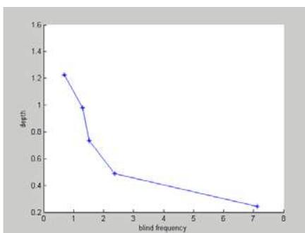
Fig. 6 Blind frequency for different depths.
