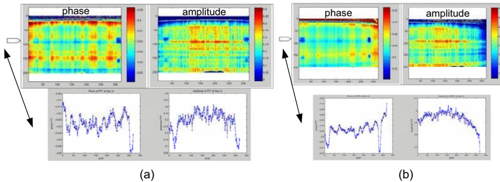
Fig. 4 Effect of orientation on phase and amplitude for *Specimen 1* with orientation of (a): 0° and (b): 20°. Second discrete frequency (0.167 Hz). Plots along image row are also shown. Phase and amplitude after normalization of temperature sequence.
