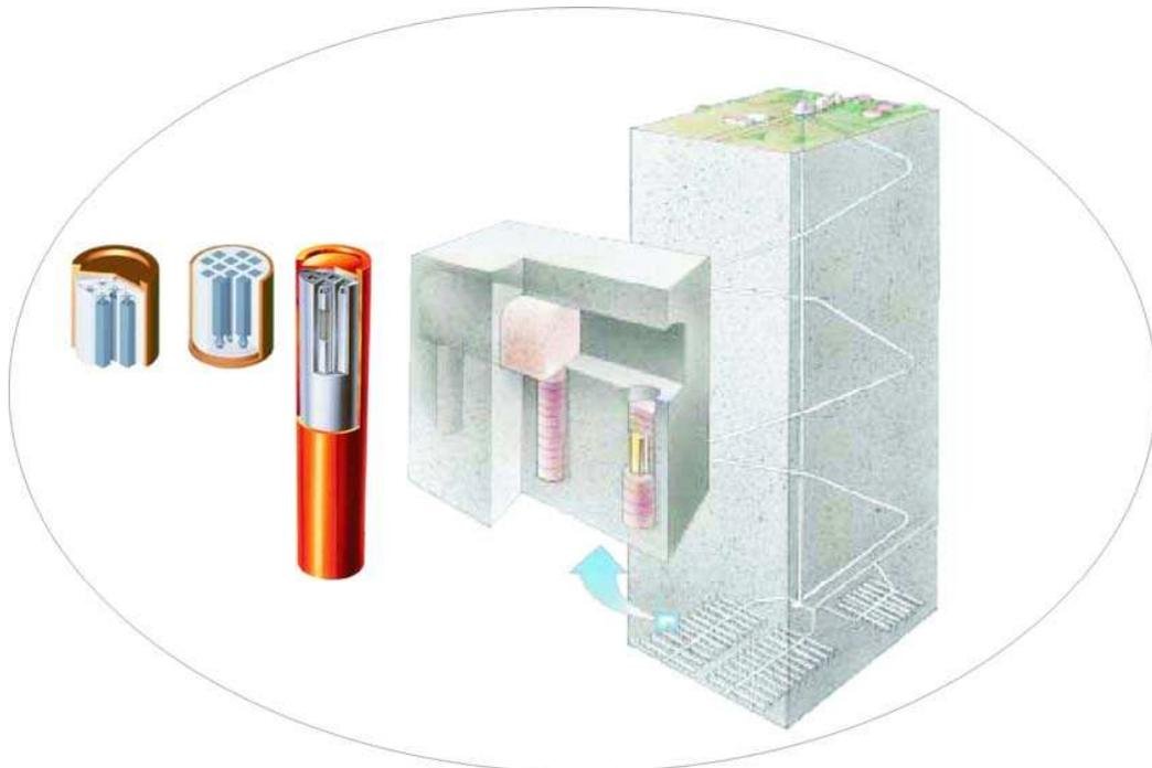
Fig. 2: Construction Plan of Copper Canisters and the Bedrock Deposit
