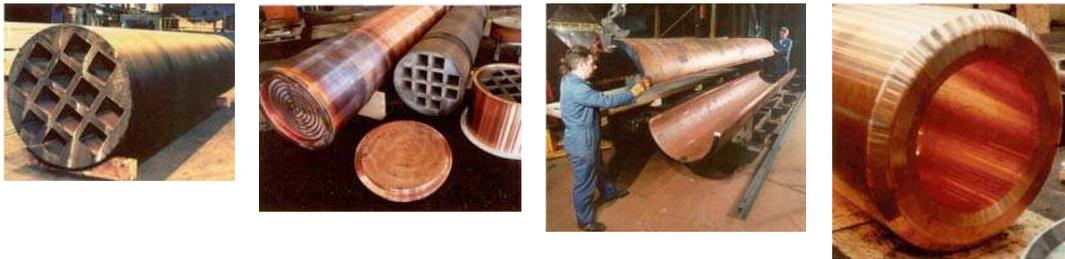
**Fig. 3: Construction of the copper canister**
